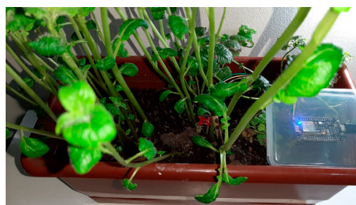
Figure 3. Prototype of ESP8266 and Sensor FC-28 in potato cultivation.
