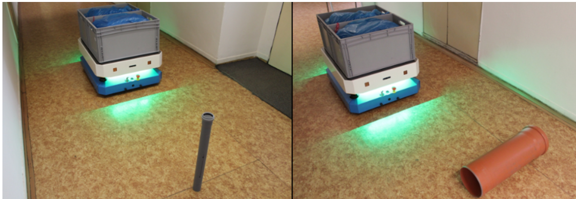
Figure 7. Experimental verification of the braking distance value.
