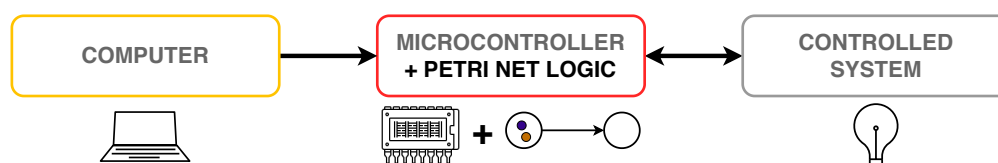
Figure 1. Basic scheme of proposed solution—Petri net’s logic in microcontroller [26].
