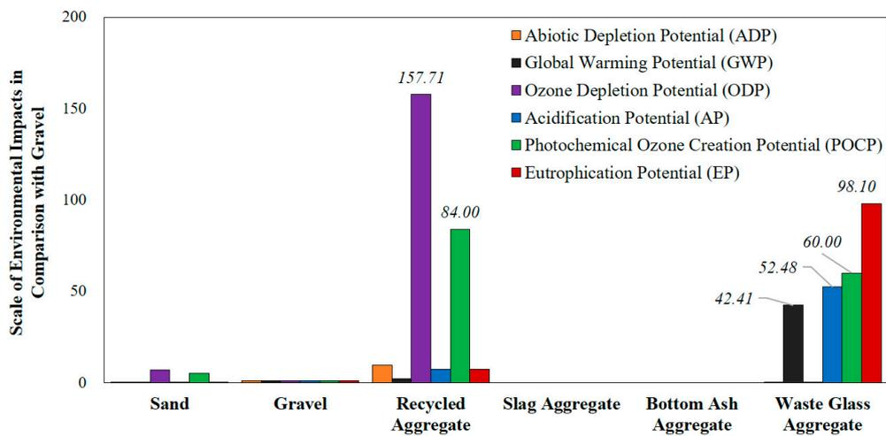
Figure 1. Scale of the Difference Between the Environmental Impact of Each Aggregate and that of Gravel.
