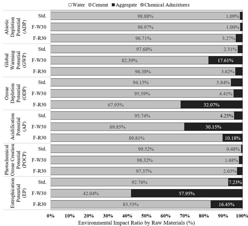
Figure 3. Environmental Impact Ratio with Respect to Raw Materials in the Standard, F-W30, and F-R30 Mixtures.
