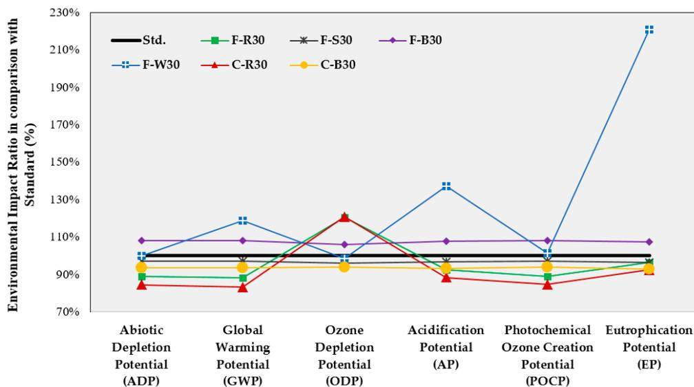
Figure 2. Environmental Impact Ratio of Each Evaluation Target in Comparison with the Standard Mixture.
