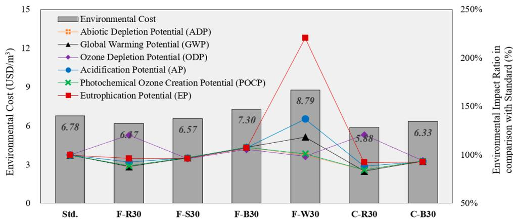
Figure 4. Environmental Cost and Environmental Impact Ratio in Comparison with Standard Mixture.
