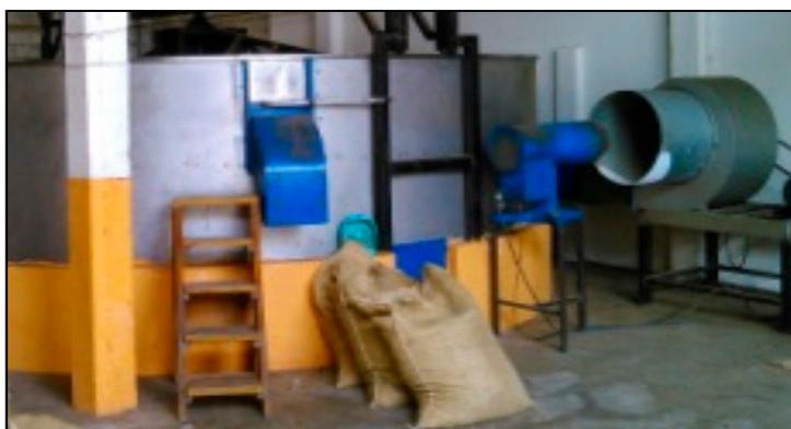
**Figure 5.** Parts of a grain dryer; drying chamber, burner, and exhaust fan.
