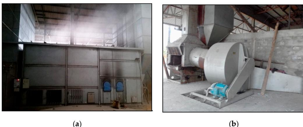
**Figure 10.** Shows two types of biomass dryers. (a) Double chamber dryer; on the left is the drying chamber and on the right is the combustion chamber. Brazilian technology, first-generation processing plant; (b) Handcrafted dryer with a drying chamber, combustion oven, ducts, and an exhaust fan in a second-generation processing plant.
