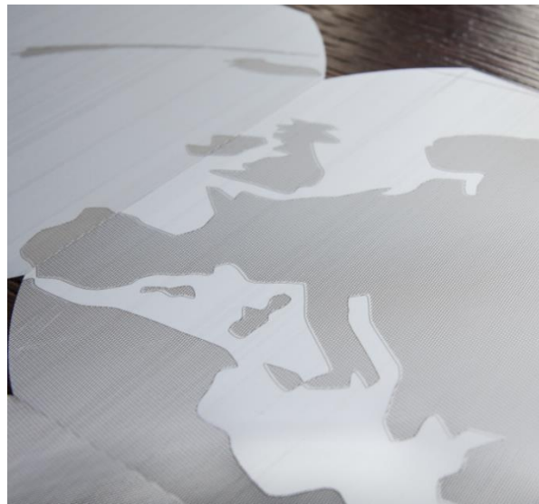
Figure 6. Large scale images of the Si wafers sub-picosecond surface hatching. Laser beam parameters: 650 fs, 343 nm, 200 kHz, 27.5 \mu J; processing parameters: 7 mm/s, 15 pattern repetitions, total processing time 1.5 h.
