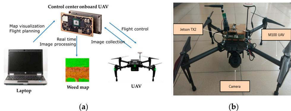
**Figure 1.** Composition of the developed system. (a) Components of the developed system. (b) Main components of the UAV system.
