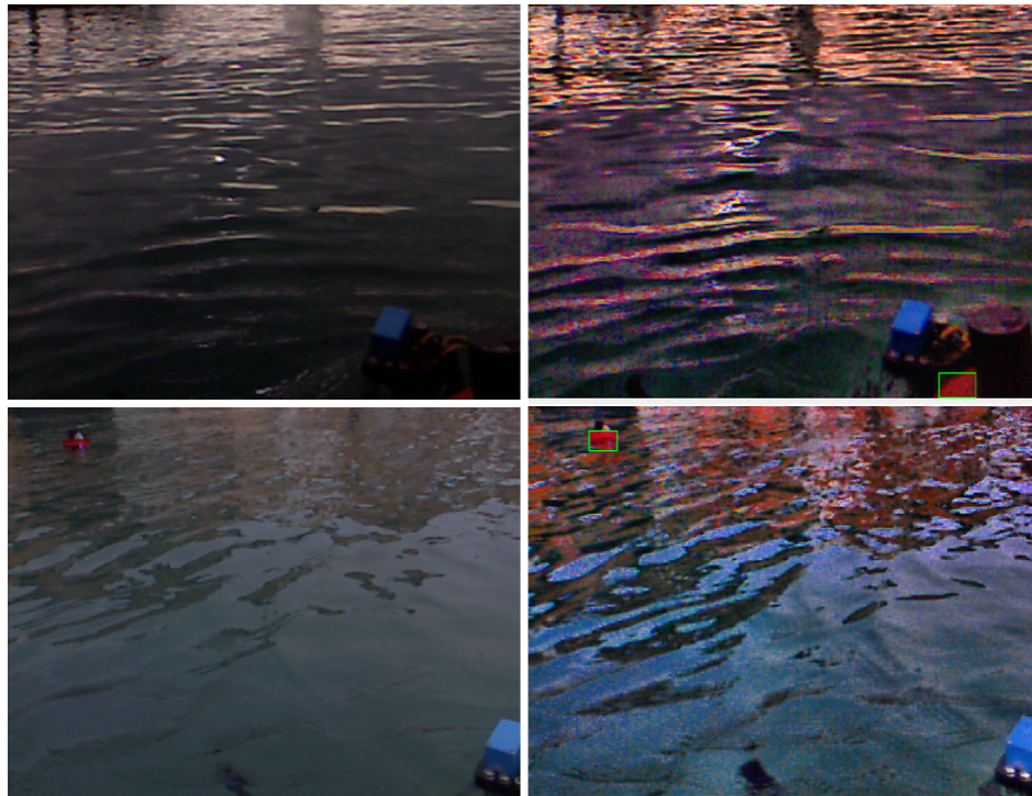
Figure 13. Two examples of aMussel top cap detection, original images captured from the Kinect camera RGB stream ( left ) and processed images ( right ). Detected aMussel bounding boxes shown in green.
