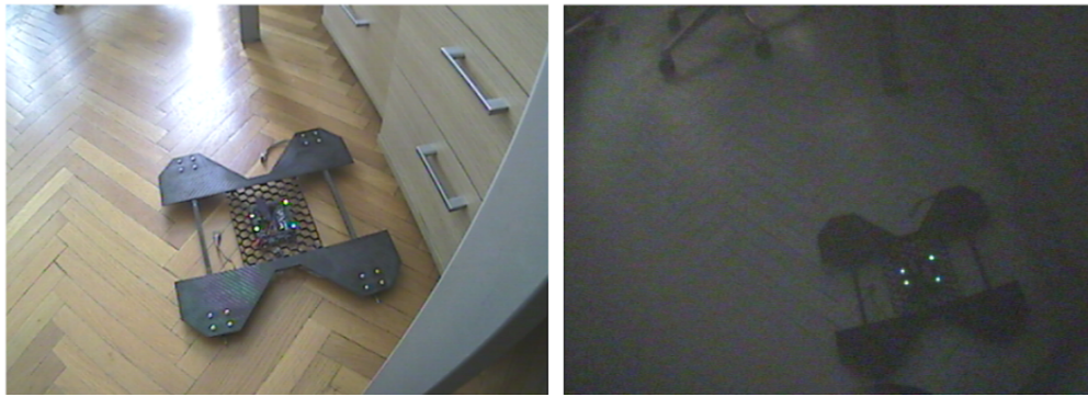
Figure 3. Example of analog camera IR filtering used in the original docking concept ( left ), no filter; ( right ) IR filtering film applied. Images are of four IR LED markers mounted on a test robot frame.
