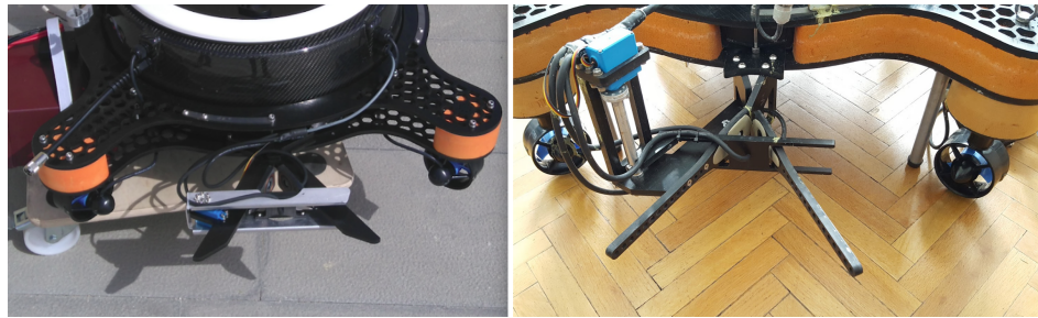
Figure 7. aPad-mounted docking mechanism comparison, initial design (left) and final design (right).
