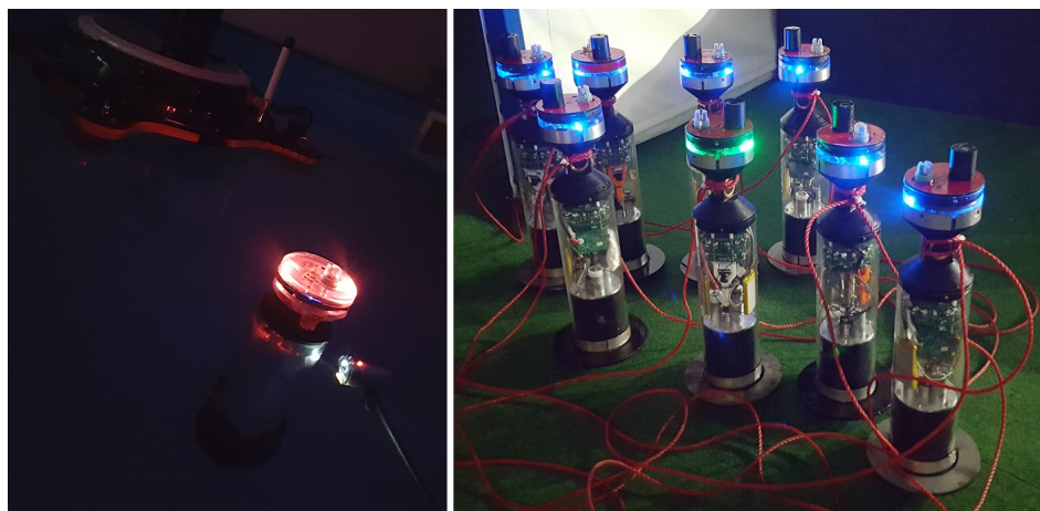
Figure 4. aMussel top cap comparison, initial version ( left ) and redesigned version ( right ).
