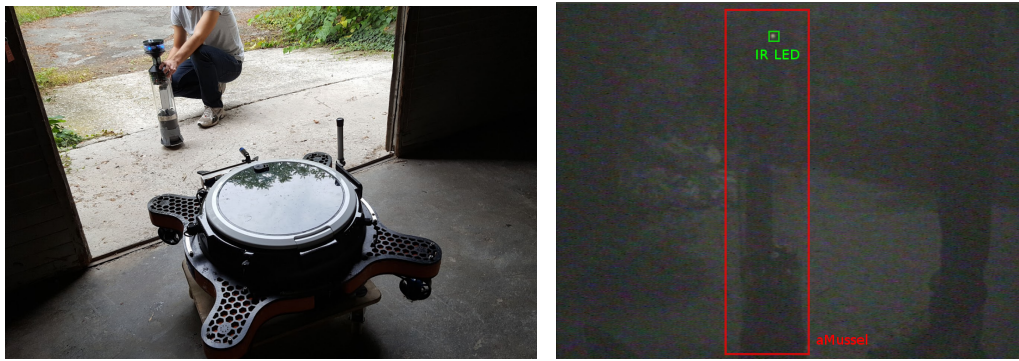
Figure 5. Initial docking vision system test for IR filtering in daylight. Only one camera and docking mechanism mounted for proof-of-concept purposes ( left ), and an example image of aMussel outdoors in ambient sunlight with IR LED in cap turned on, viewed through an analog camera with IR filter applied ( right ).
