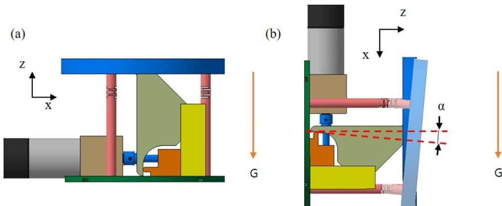
**Figure S2.** Examples of the SMFH orientation with the gravity that acts along (a)  $-z$ -direction and (b)  $-x$ -direction.
