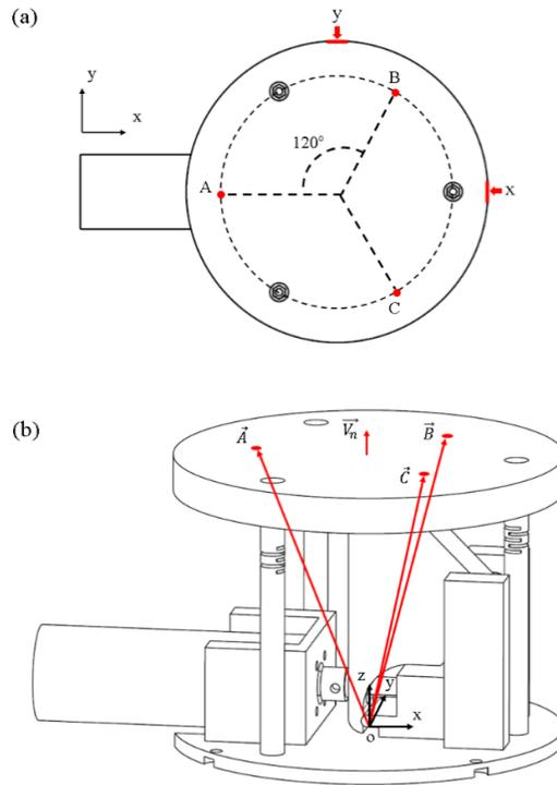
**Figure S1.** (a) Five spots for obtaining displacement data and (b) notation of coordinate and vector directions.
