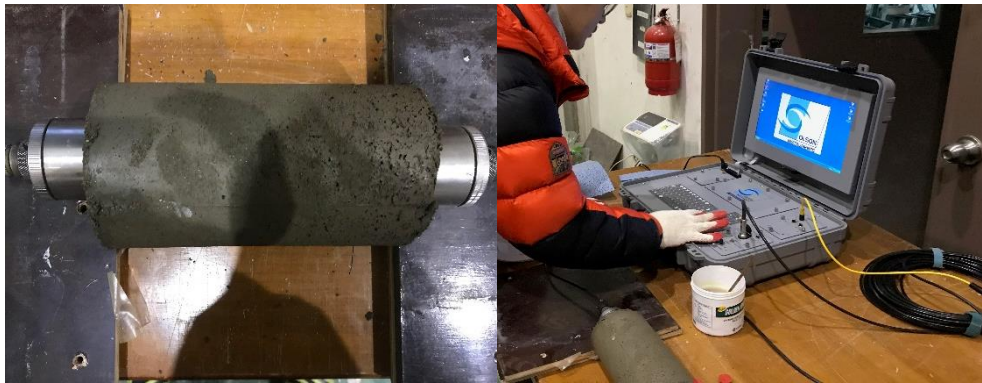
Figure 2. Experiment of ultrasonic pulse velocity method.
