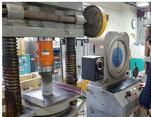
Figure 3. Testing method for compressive strength of molded concrete cylinders.
