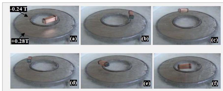
**Figure 8.** Laboratory scale tests with the PMG-system of a circular type (a–f—consecutive video frames of the HTSC-Sabot counterclock-wise moving).
