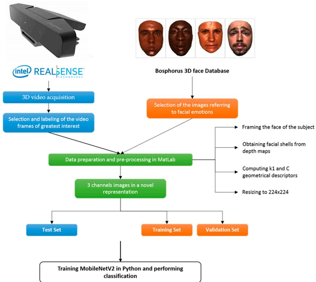
**Figure 2.** Scheme of the proposed methodology. Blue refers to the sensor, from acquisitions to test set, orange refers to the Bosphorus DB, and green to the common operations of data preparation and pre-processing.
