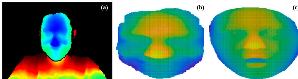
**Figure 1.** Depth map in output from the 3D sensor (a), the same data elaborated in MatLab (b), and the shell of a Bosphorus DB image (c).
