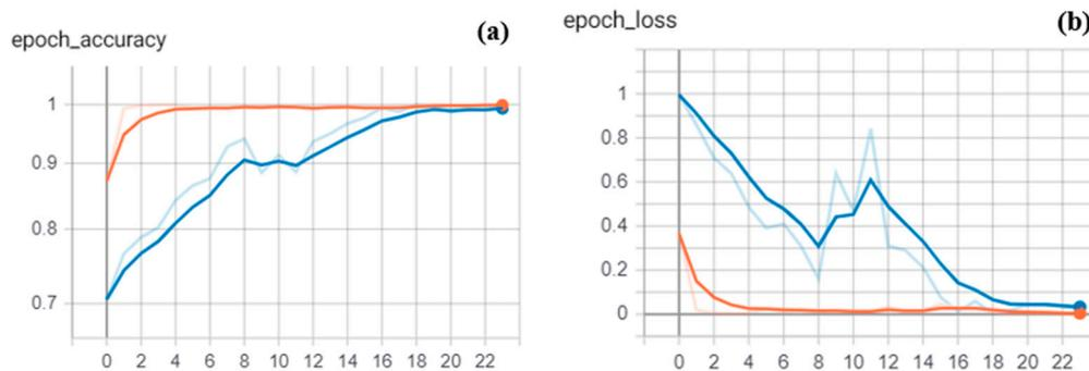
**Figure 4.** Tensorboard diagrams of accuracy (a) and loss (b) on the training and validation dataset, respectively orange and blue, over training epochs. The training and validation accuracy gradually increase to around 1, whereas the training and validation loss converges to 0.01 after 23 epochs. Overfitting does not occur during the training.
