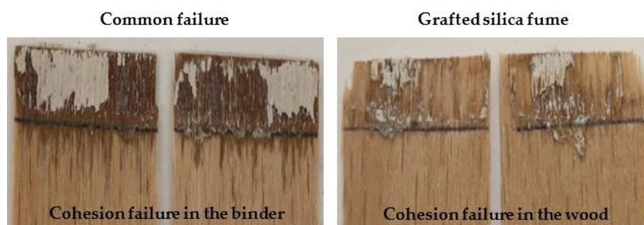
Figure 4. Fractured surface of the geopolymer binder mixed with various additives using the ABES instrument.
