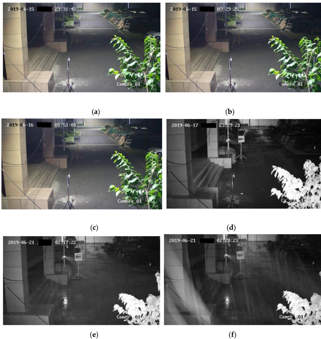
Figure 8. Samples of different visibility representative images acquired in actual measurements. The measured values are (a) 10,000 m, (b) 8007 m, (c) 5181 m, (d) 2250 m, (e) 861 m, (f) 177 m.
