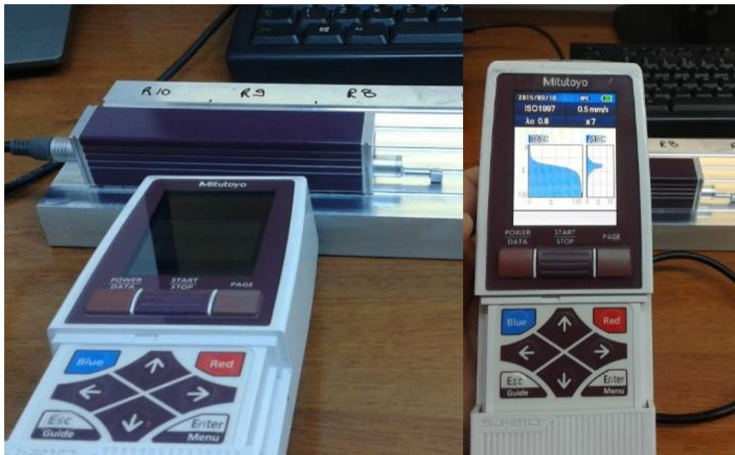
Figure 6. The measurements made with Mitutoyo SURFTEST SJ-210.
