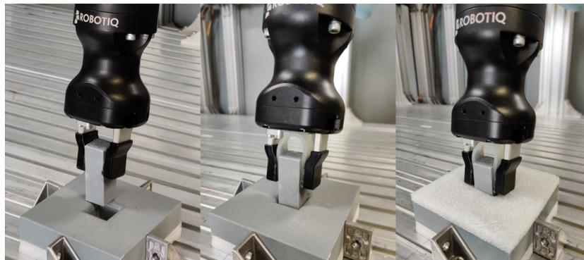
**Figure 8.** High, medium, and low-stiffness environments (left to right).
