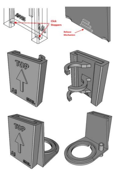
**Figure 1.** FreeCAD renderings of the fastening mechanism on the sheath (**top left**), releasing mechanism on the slider (**top right**), clip system from the back (**middle left**), clip system with hose holder tool from the front (**middle right**), redesigned clip system for the cyclone sampler from the back (**bottom left**), and redesigned clip system for the cyclone sampler from the front (**bottom right**).
