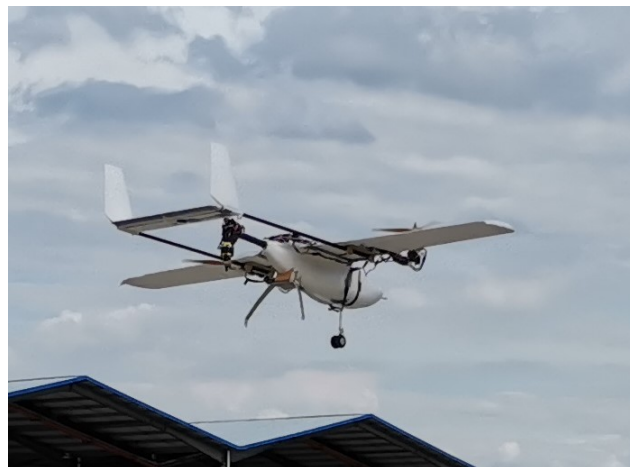
Figure 12. Experimental scene of the tilt tri-rotor UAV in the hover mode.
