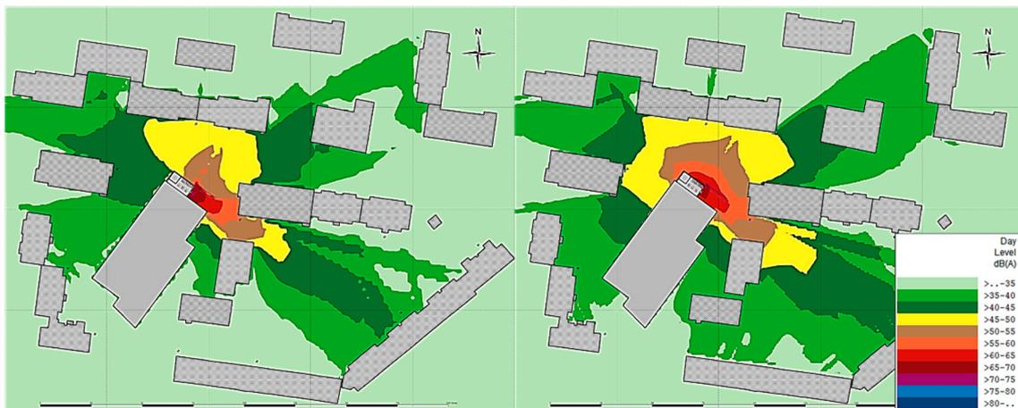
**Figure 7.** Scenario 3 with a sloped acoustic barrier and higher height—Lday with all noise sources (left: 4 m, right: 10 m).
