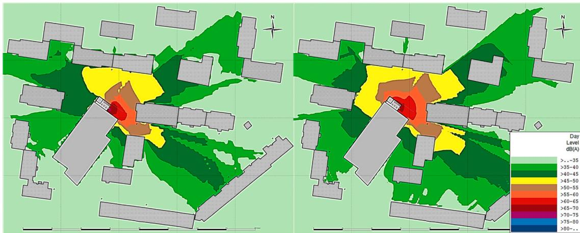
**Figure 6.** Scenario 2 with acoustic barrier of 2.3 m—Lday with all noise sources (left: 4 m, right: 10 m).
