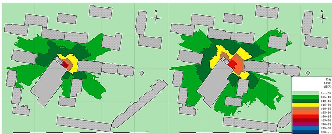
**Figure 9.** Scenario 5 with a supply ramp inside a construction and acoustic barriers on the roof—Lday with all noise sources (left: 4 m, right: 10 m).
