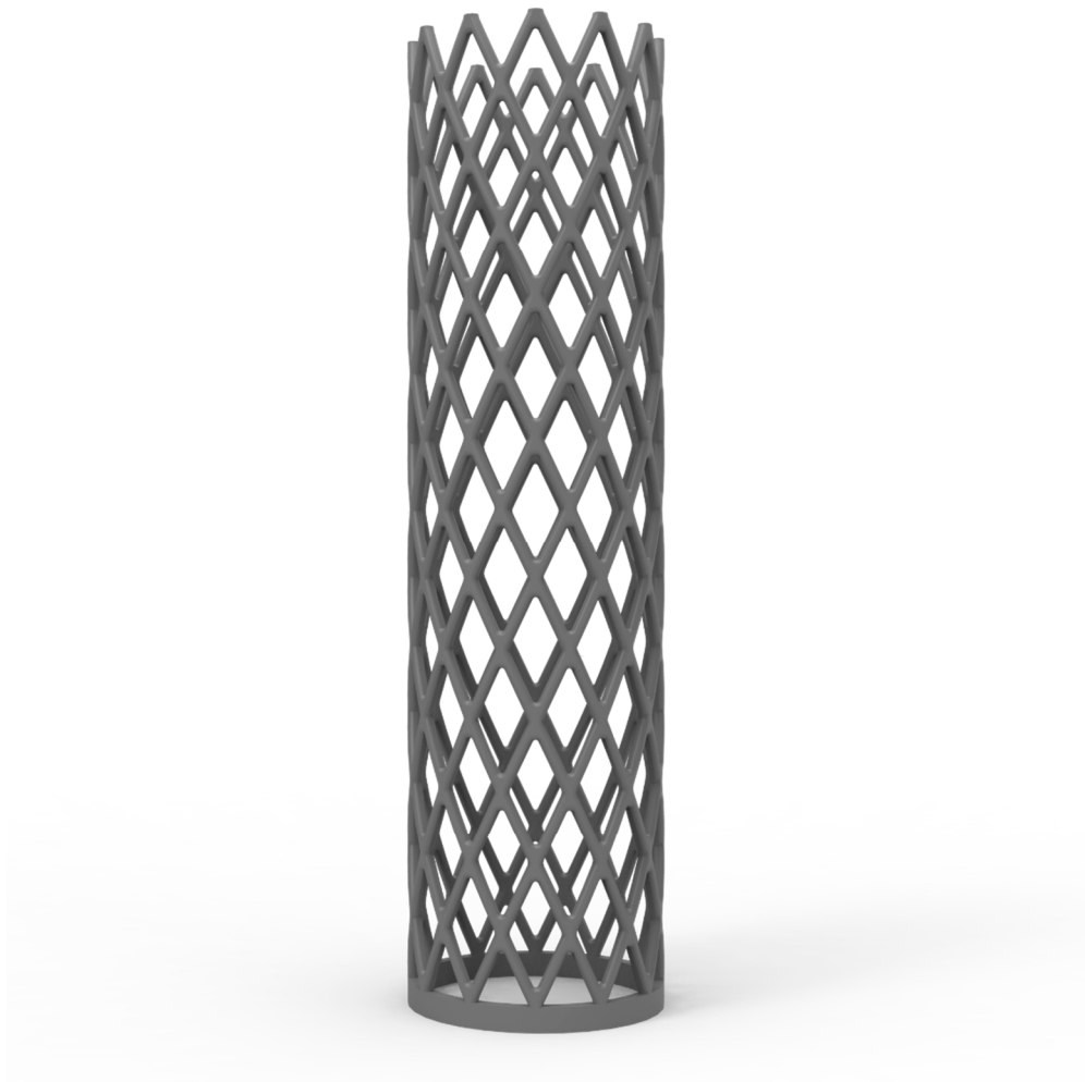
Figure 4. Rendering of the net structure with homogenized nodes through rounding from CAD.
