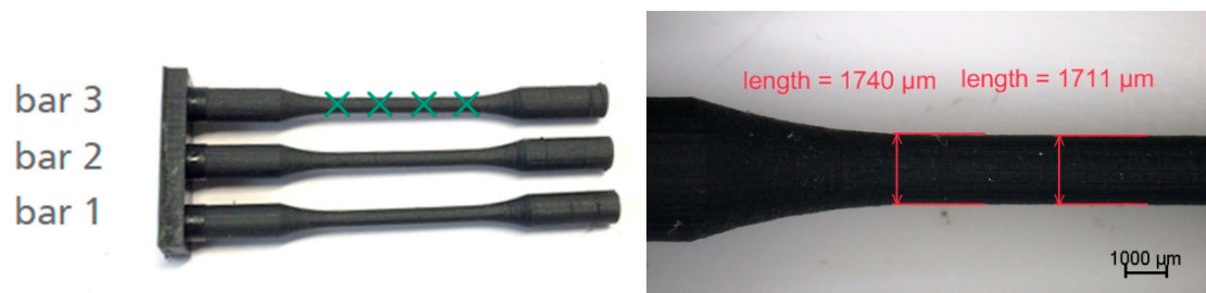
Figure 5. Round tension bars with exemplary markings of measuring points.
