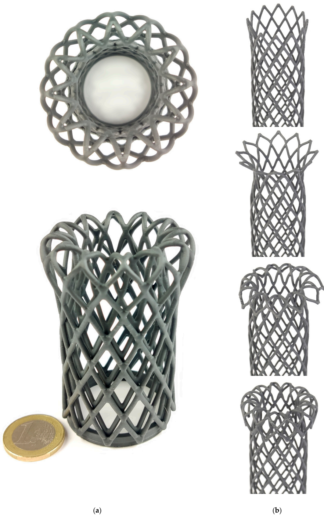
Figure 17. Additively manufactured everted tubular net structure with homogenized nodes: everted over the entire length in top and side view (a) and in different stages of the everting process from top to bottom (b) (captured in reverse transformation).
