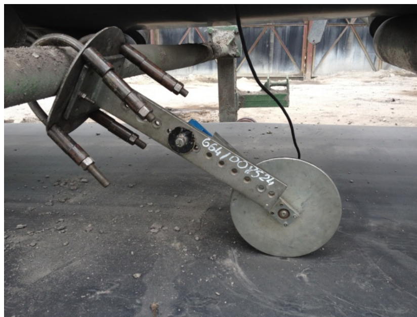
Figure 3. Encoder installed on the belt conveyor.
