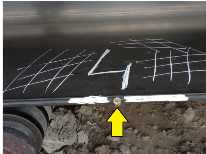
Figure 4. One of the marked neodymium magnets attached to the conveyor belt.
