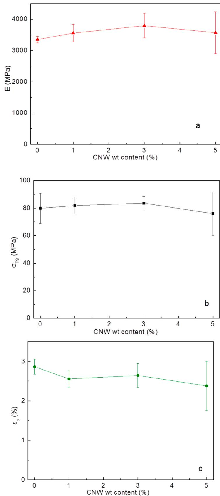
**Figure 10.** Diagrams of (a) modulus of elasticity (E), (b) tensile strength ( $\sigma_{TS}$ ) and (c) strain at break ( $\epsilon_b$ ) as a function of the weight fraction of the nano-additive into the samples.
