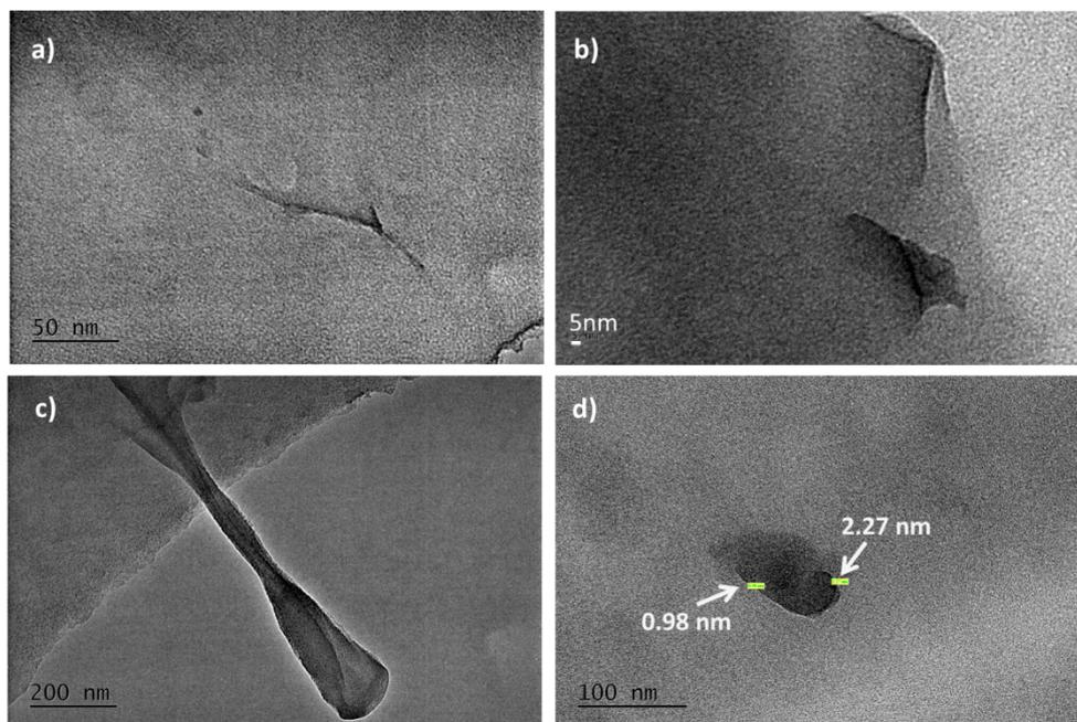
Figure 8. Transmission electron microscopy (TEM) images of PS-CNWs-3% nanocomposite (a–d).
