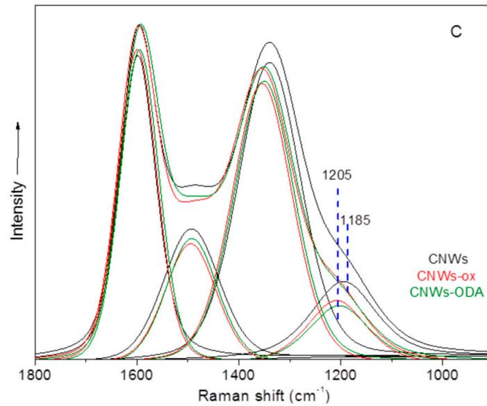
**Figure 3.** (a) Raman spectra of CNWs, CNWs-ox and CNWs-ODA samples; (b) normalized spectra; and (c) spectra analyzed to Gaussian profiles.
