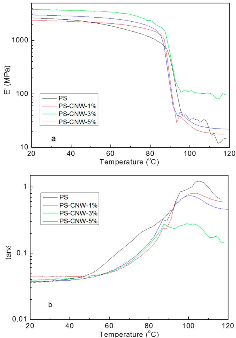
**Figure 11.** Diagrams of (a) storage modulus ( $E'$ ) and (b) loss factor ( $\tan\delta$ ) of the nanocomposites and the pristine material.
