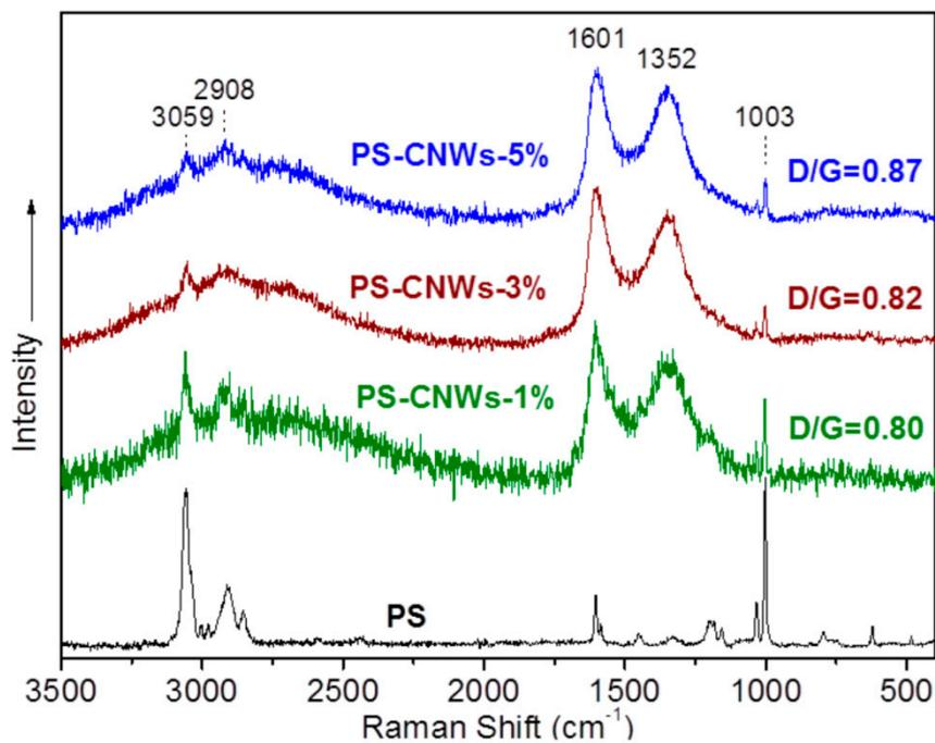
Figure 7. Raman spectra of neat PS, PS-CNWs-1%, PS-CNWs-3% and PS-CNWs-5% samples.
