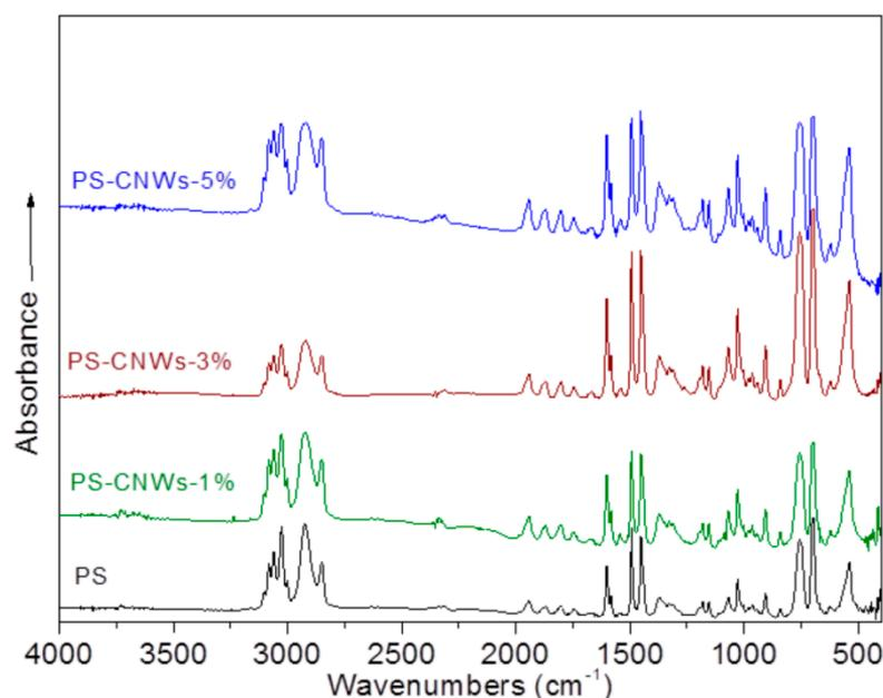
**Figure 5.** Fourier-transform infrared (FT-IR) spectra of samples: neat polystyrene (PS), PS-CNWs-1%, PS-CNWs-3% and PS-CNWs-5% samples.
