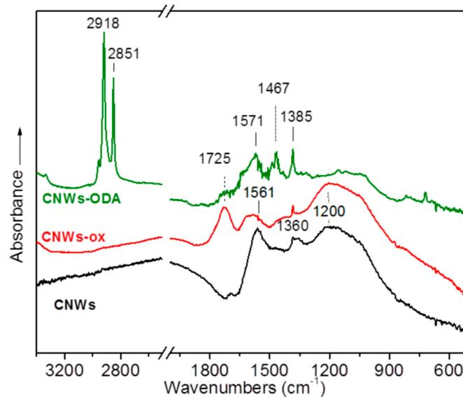
**Figure 1.** FT-infrared spectra of samples: carbon nanowires (CNWs), oxidized CNWs (CNWs-ox) and CNWs-ODA.
