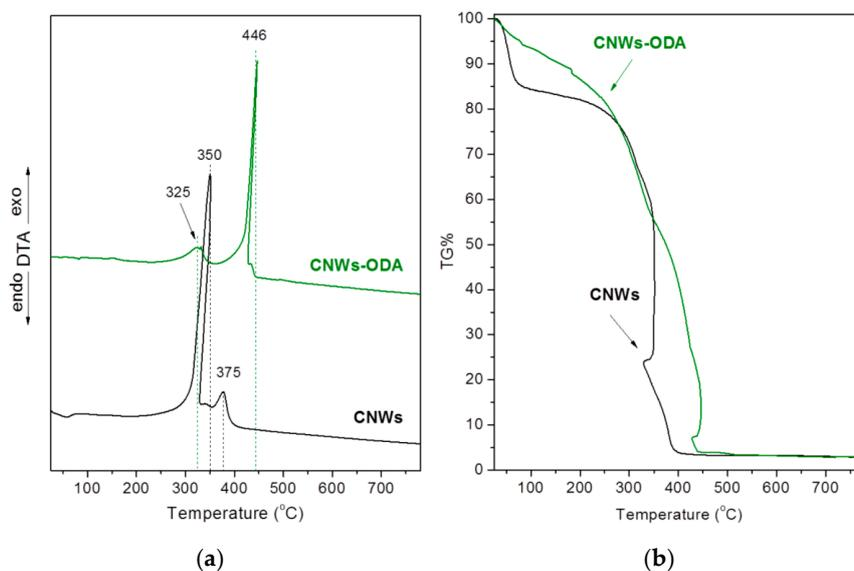
**Figure 2.** Differential thermal (DTA) (a) and thermogravimetric analysis (TGA) (b) curves of CNWs and CNWs-ODA samples.
