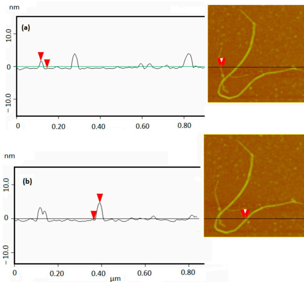
**Figure 4.** Images from atomic force microscopy (AFM) of the CNWs sample (right) and its topographical profile in (a,b).
