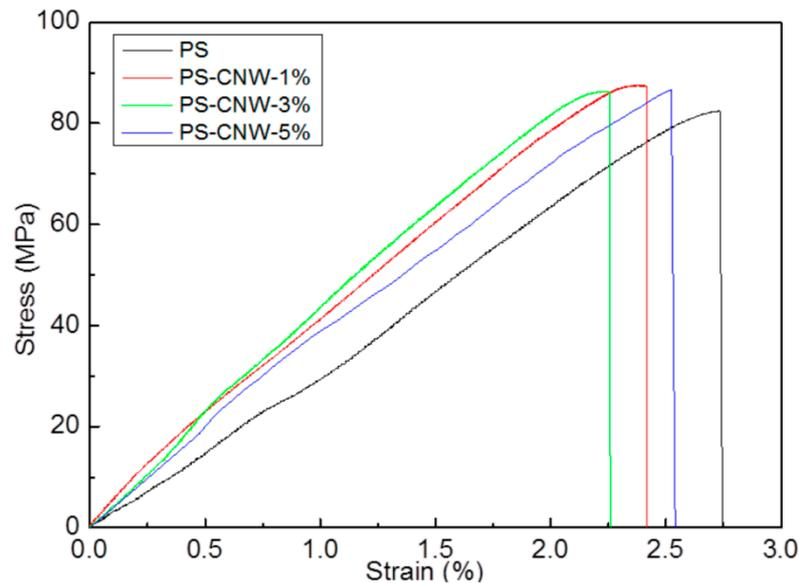
**Figure 9.** Stress–strain diagrams for the nanocomposite samples as well as for the pristine polymer.
