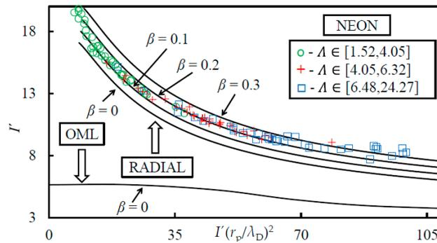
**Figure 2.** Neon plasma Sonin plot for the normalized probe potential  $y_{SP} = 25$ . Experimental data for the neon plasma: green circles for  $1.52 \leq \Lambda \leq 4.05$ , red crosses for  $4.05 \leq \Lambda \leq 6.32$  and blue squares for  $6.48 \leq \Lambda \leq 24.27$ . In solid lines, the orbital and radial theoretical curves are shown.
