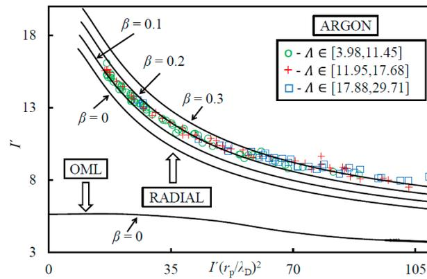
**Figure 1.** Argon plasma Sonin plot for the normalized probe potential  $y_{SP} = 25$ . Experimental data for the argon plasma: green circles for  $3.98 \leq \Lambda \leq 11.45$ , red crosses for  $11.95 \leq \Lambda \leq 17.68$  and blue squares for  $17.88 \leq \Lambda \leq 29.71$ . In solid lines, the orbital and radial theoretical curves are shown.
