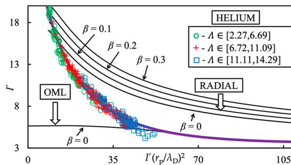
**Figure 3.** Helium plasma Sonin plot for the normalized probe potential  $y_{SP} = 25$ . Experimental data for the helium plasma: green circles for  $2.27 \leq \Lambda \leq 6.69$ , red crosses for  $6.72 \leq \Lambda \leq 11.09$  and blue squares for  $11.11 \leq \Lambda \leq 14.29$ . In solid lines, the orbital and radial theoretical curves are shown. In purple bold line, the fitting curve for the experimental helium plasma Sonin plot points is shown.
