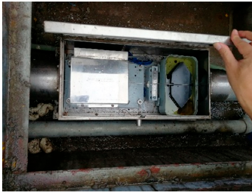
Figure 6. Layout of tension wire alignment device observing horizontal displacements.
