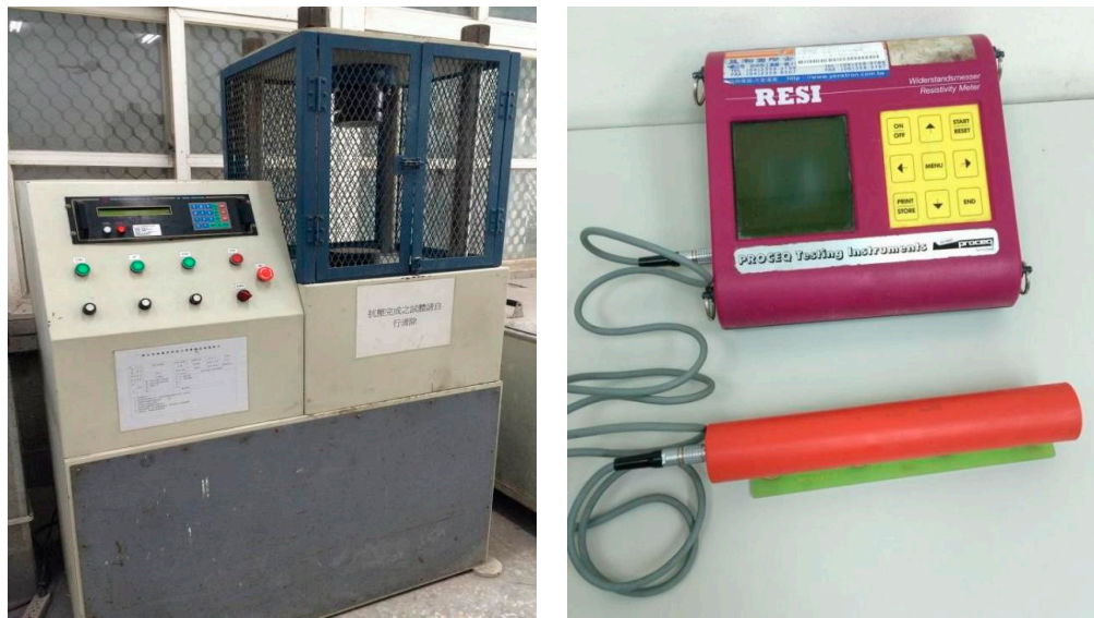
Figure 1. Test equipment. (a) Compressive strength-testing machine. (b) Four-pole resistance-measuring instrument.
