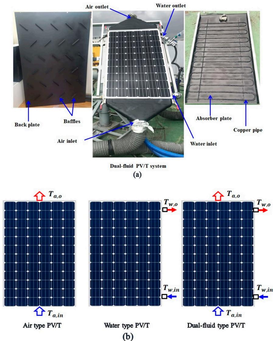
Figure 1. (a) Experiment setup and (b) flow schemes.
