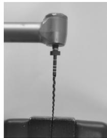
**Figure 2.** Device for torsional resistance tests.
