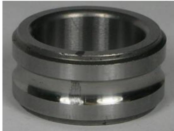
**Figure 7.** The rolling bearing with inner race fault.
