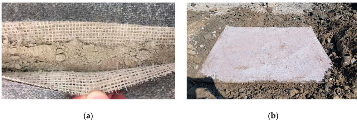
Figure 1. Concrete mat: (a) composition of a concrete mat; (b) field application example.
