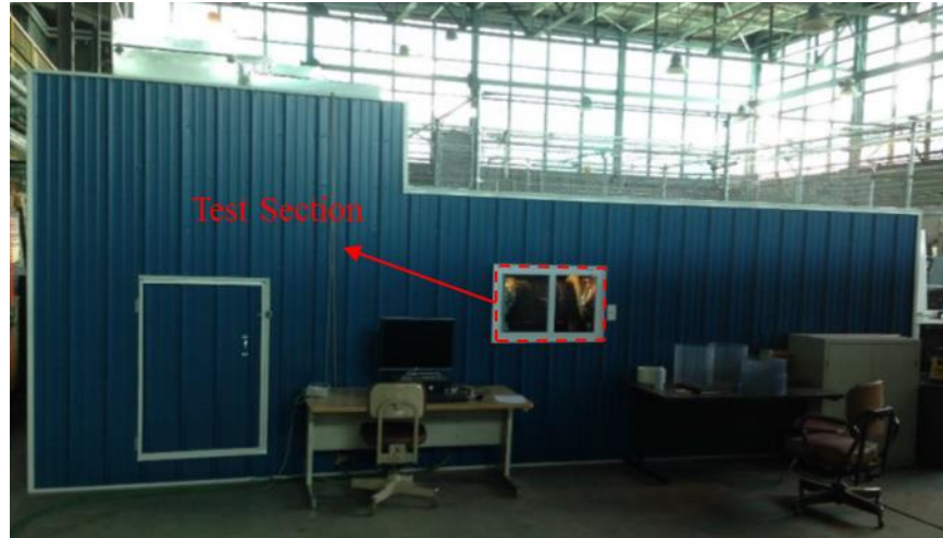
Figure S1. A walk-in freezing room connected to a wind tunnel that is used for forming snow in controlled temperatures.
