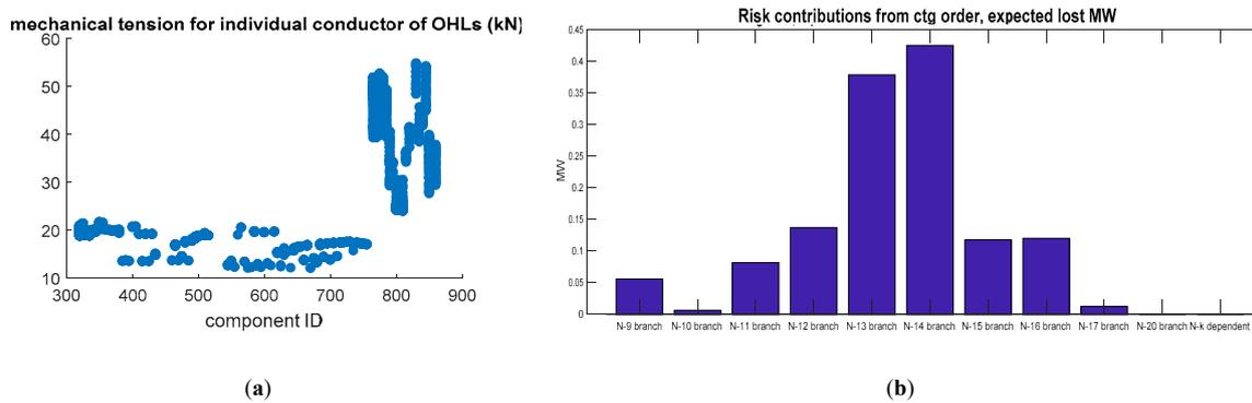
**Figure 11.** (a) Mechanical tension in kN for medium voltage (MV) MV and high voltage (HV) lines, (b) Contributions to total risk of each contingency category, case EM4.
