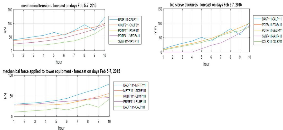
**Figure 7.** Ice thickness in mm (**top right diagram**), mechanical tension (**top left diagram**) and mechanical load on tower equipment in kN (**bottom left diagram**) in the first 10 h of the forecasting interval.
