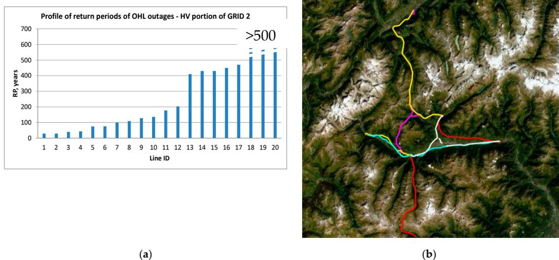
**Figure 4.** (a) List of overhead lines (OHLs) with increasing RPs—EN 50341 indications for extreme values distribution, (b) Georeferenced map of OHLs with colors indicating increasing values of return periods (from magenta to white)—extreme values evaluated via Std EN 50341-2-13.
