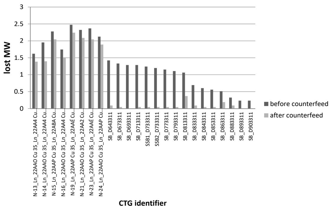
**Figure 12.** Bar diagram of the LOL impact of the contingencies before and after the new counterfeed, severe wet snow event EM3-P1.
