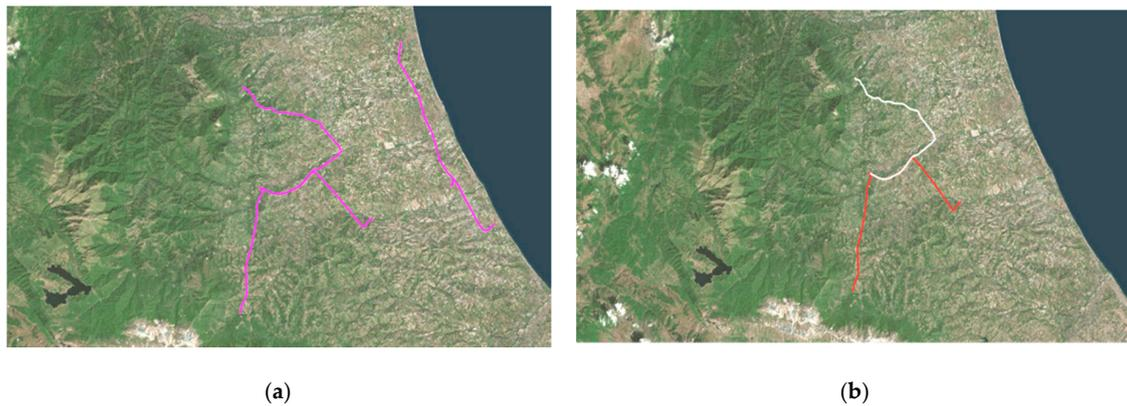
**Figure 8.** Geolocalization of critical components for severe wet snow (a) and moderate wet snow storm (b).
