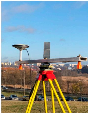
**Figure 4.** Second test setup. Huawei P30 Pro mounted in vertical position.
