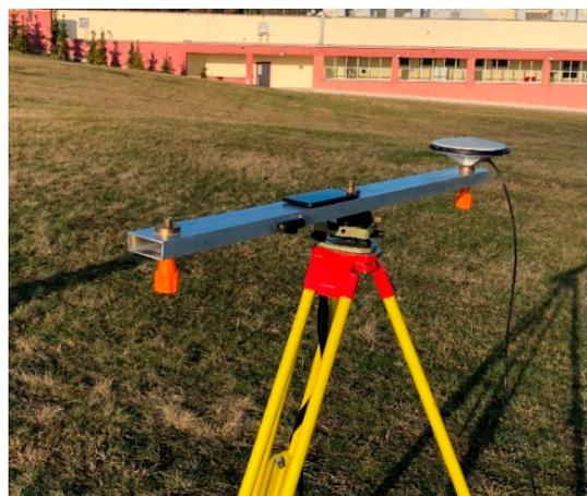
**Figure 5.** Third test setup. Huawei P30 Pro mounted in a horizontal position.
