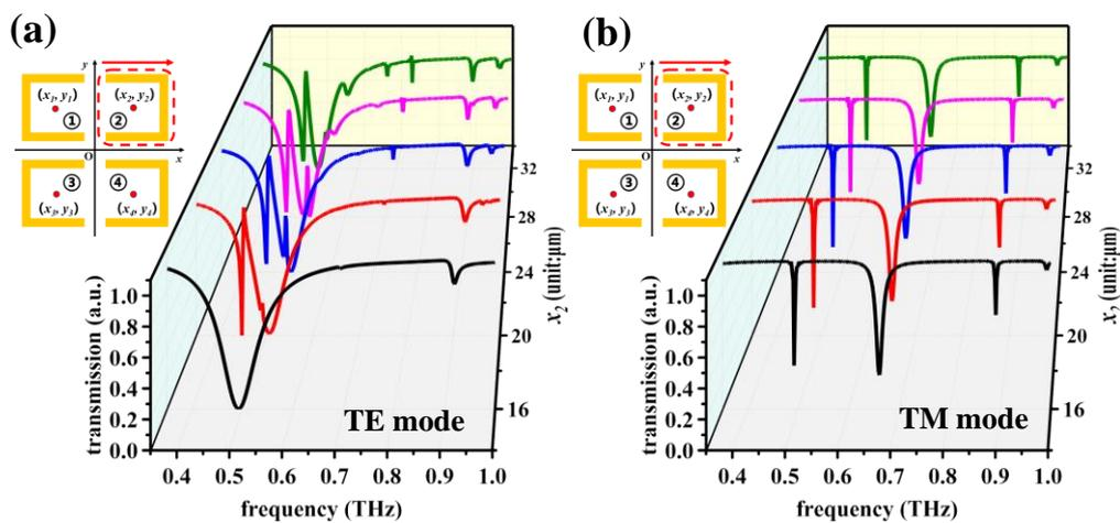
**Figure 6.** Simulated transmission spectra of the RTM device obtained by moving the SRR-2 meta-atom along positive  $x$ -axis direction in (a) TE and (b) TM modes.
