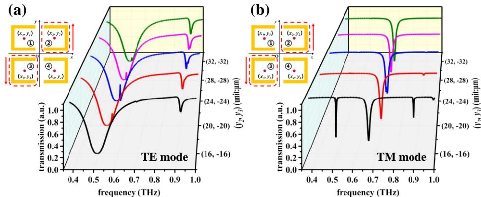
**Figure 9.** Simulated transmission spectra of RTM device obtained by moving the SRR-2 and SRR-3 meta-atoms along positive and negative  $y$ -axis directions in (a) TE and (b) TM modes, respectively.
