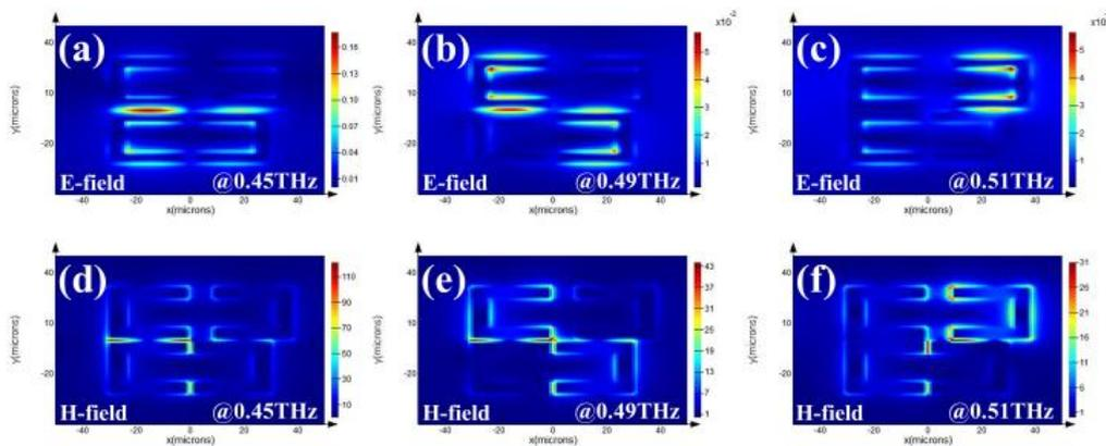
Figure 7. (a–c) E-field and (d–f) H-field distributions of the RTM device with  $x_2 = 24 \mu\text{m}$  in TE mode.
