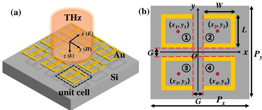
**Figure 1.** (a) Schematic drawing of the proposed reconfigurable terahertz (THz) metamaterial (RTM) device with four split-ring resonator (SRR) meta-atoms; (b) The geometric parameters of four SRR meta-atoms. The geometric dimensions are:  $W = 30 \mu\text{m}$ ,  $L = 30 \mu\text{m}$ ,  $G = 2 \mu\text{m}$  and  $P_x = P_y = 100 \mu\text{m}$ . The reference points are  $(x_1, y_1) = (-16, 16)$ ,  $(x_2, y_2) = (16, 16)$ ,  $(x_3, y_3) = (-16, -16)$  and  $(x_4, y_4) = (16, -16)$ .
