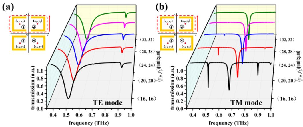
**Figure 3.** Simulated transmission spectra of the RTM device obtained by moving the SRR-1 and SRR-2 meta-atoms along positive  $y$ -axis direction in (a) TE and (b) TM modes.
