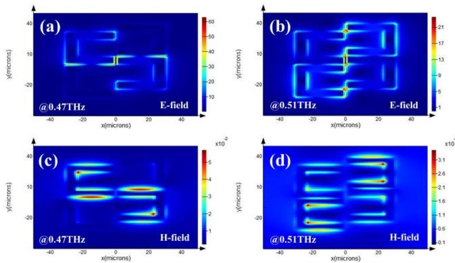
**Figure 5.** (a,b) E-field and (c,d) H-field distributions of the RTM device with  $(y_2, y_4) = (24, -8) \mu\text{m}$  in TE mode.
