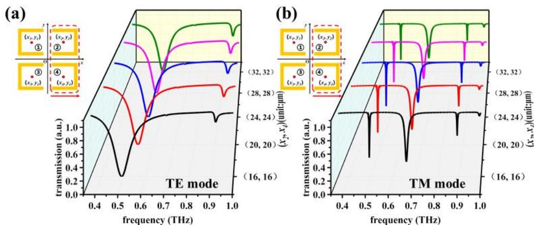
**Figure 2.** Simulated transmission spectra of the RTM device obtained by moving the SRR-2 and SRR-4 meta-atoms along the positive  $x$ -axis direction in (a) transverse electric (TE) and (b) transverse magnetic (TM) modes.
