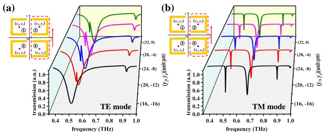
**Figure 4.** Simulated transmission spectra of the RTM device obtained by moving the SRR-2 and SRR-4 meta-atoms along positive  $y$ -axis direction in (a) TE and (b) TM modes.
