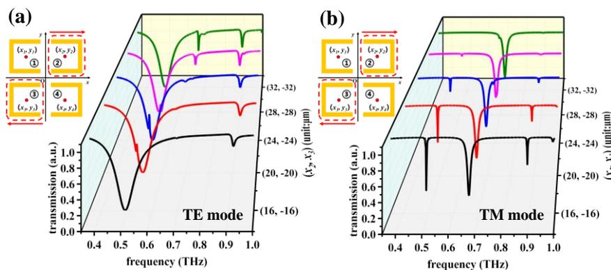
Figure 8. Simulated transmission spectra of the RTM device obtained by moving the SRR-2 and SRR-3 meta-atoms along positive and negative  $x$ -axis directions in (a) TE and (b) TM modes, respectively.
