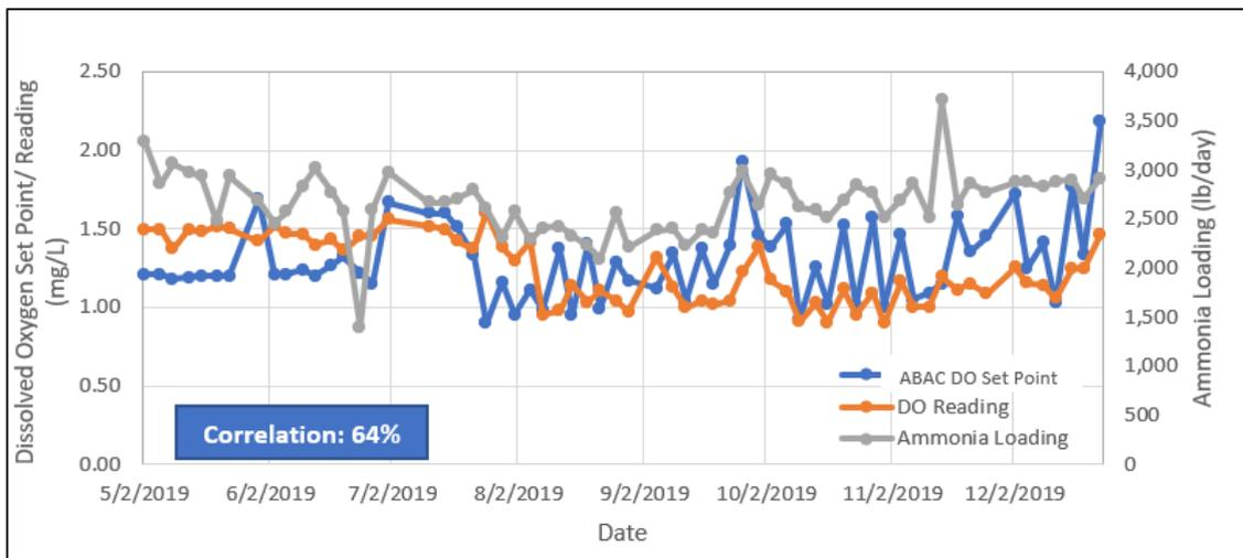
**Figure A6.** Average daily ammonia loading measured in pounds per day (lbs/day) as compared to ABAC DO set point and measured DO in aeration basins for System B. There is 45% correlation between the ABAC set DO point and the measured value.
