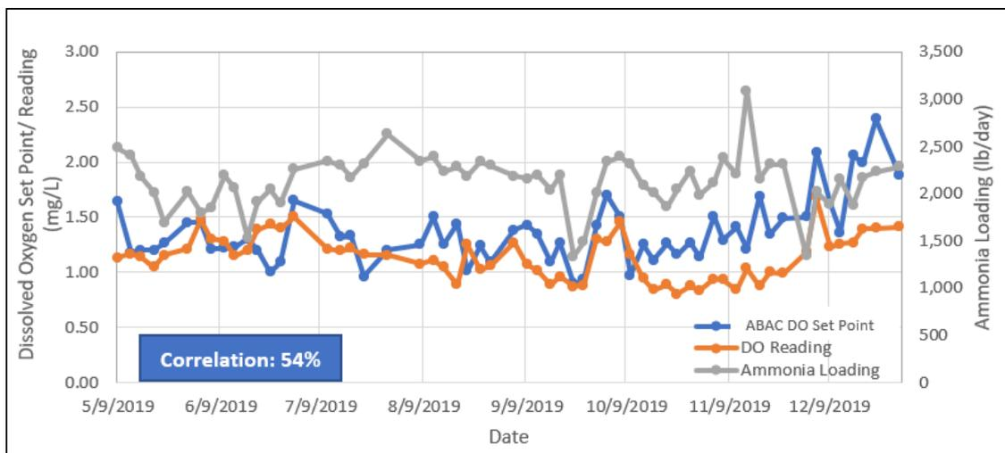
Figure A5. Average daily ammonia loading measured in pounds per day (lbs/day) as compared to ABAC dissolved oxygen (DO) set point and measured DO in aeration basins for System A. There is 54% correlation between the ABAC set DO set point and the measured value.
