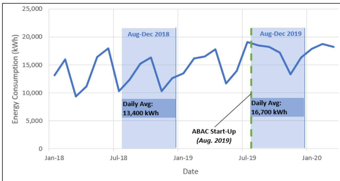
**Figure 2.** Average daily energy consumption in kWh, as measured by existing meter on aeration blowers. August through December 2018 showed a daily average energy consumption of 13,400 kWh, while the same months in 2019 showed 16,700 kWh.
