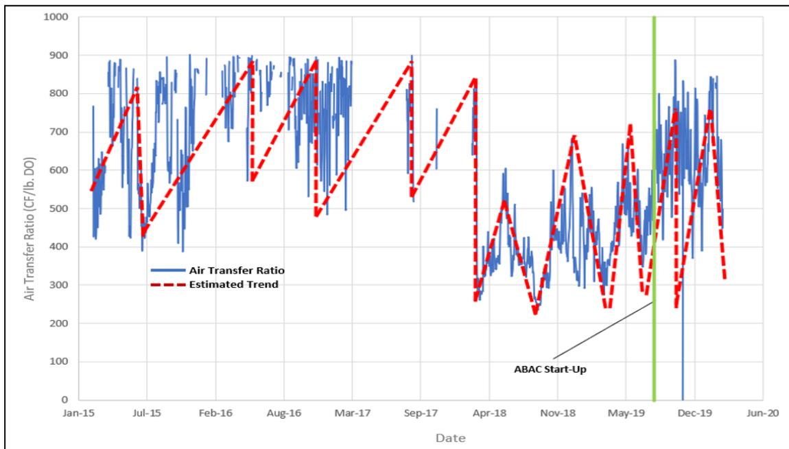
**Figure 6.** Air transfer ratio calculated in cubic feet per pound of dissolved oxygen for System B, Train 3, per Equation (2).
