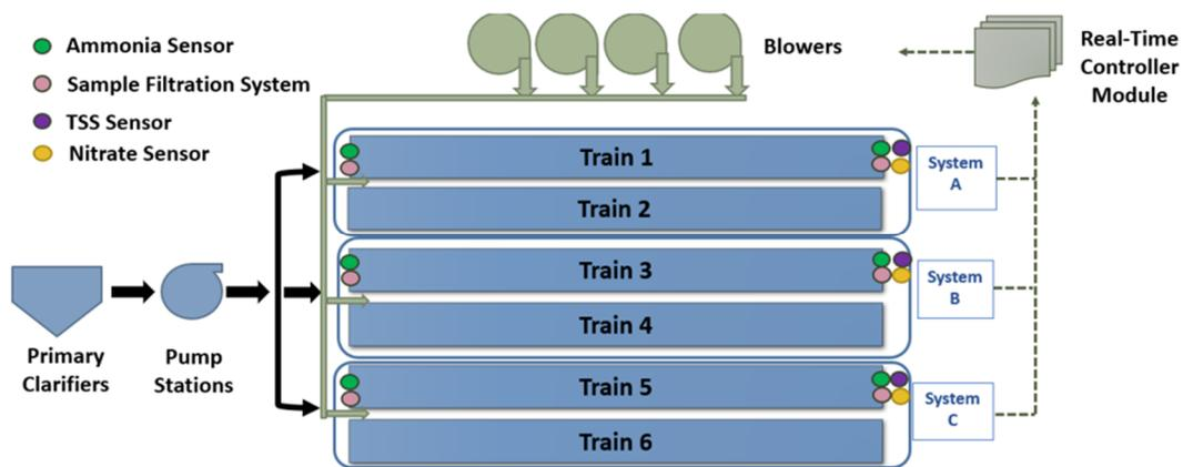
**Figure 1.** RP-1 aeration treatment process schematic with locations of an Ammonia-Based Aeration Control (ABAC) system components. Results.
