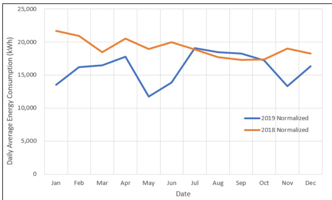
**Figure 8.** Average daily energy consumption in kWh for normalized data.
