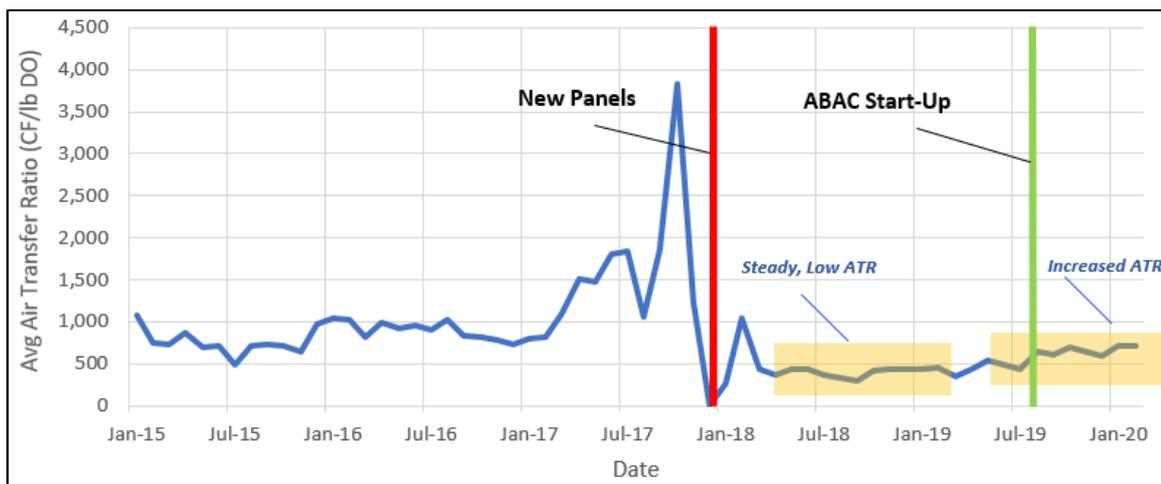
**Figure 7.** Monthly average air transfer ratio calculated in cubic feet per pound of dissolved oxygen for System B, Train 3, per Equation (2).
