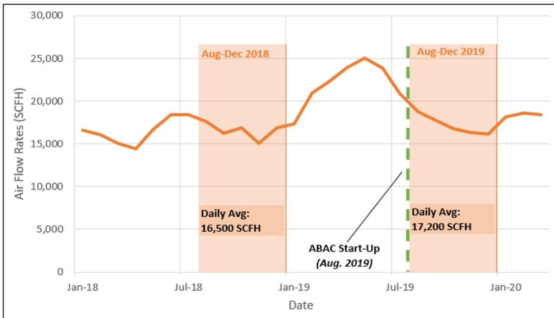
**Figure 3.** Average daily air flow rate in standard cubic feet per hour (SCFH), as measured by existing meter on aeration blowers. August through December 2018 showed a daily average air flow rate of 16,500 kWh, while the same months in 2019 showed 17,200 kWh.
