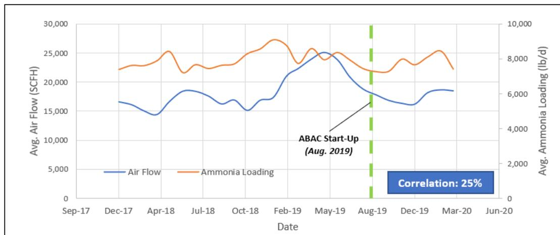
**Figure A4.** Average daily ammonia loading measured in pounds per day (lbs/day) as compared to average daily air flow rate measured in standard cubic feet per hour (SCFH). Using a correlation function, a 25% correlation is found between both parameters.
