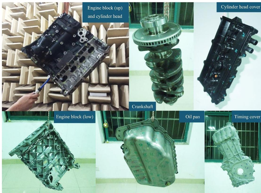
Figure 4. Modal experiments of components.
