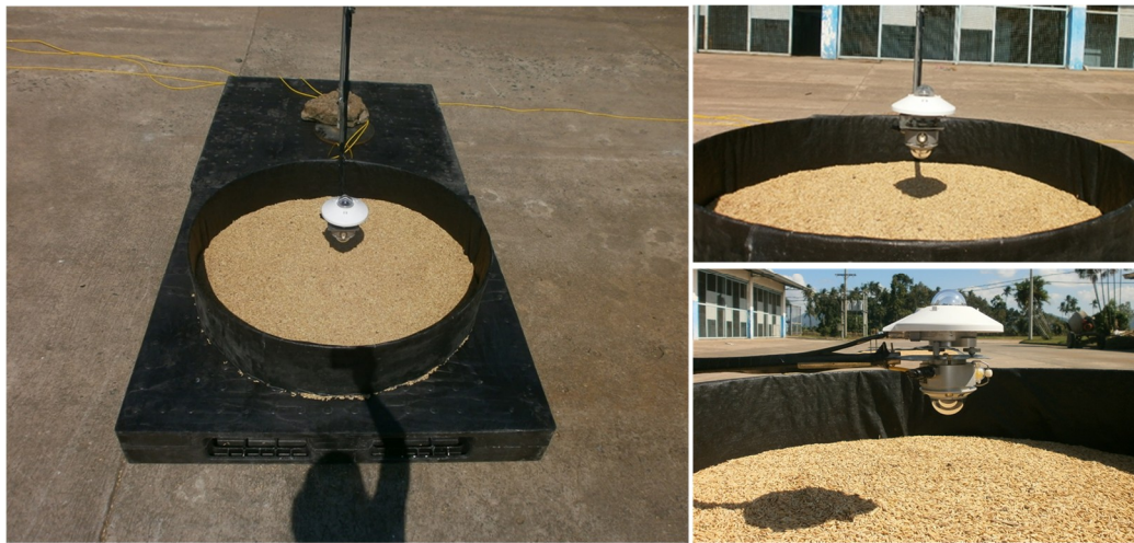
Figure 3. Setup of the pyranometers for measuring albedo at International Rice Research Institute (IRRI) in Los Baños, Republic of the Philippines (14°9′55″ N, 121°15′37″ E).
