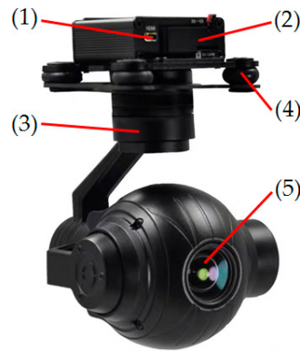
Figure 3. 3-axis gimbaled camera. (1) the output port of the video stream; (2) the embedded stabilization controller; (3) the brushless DC motor with magnetic rotary encoder; (4) the vibration damper; (5) the camera.
