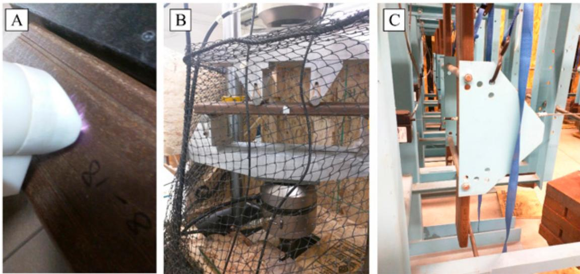
**Figure 2.** Experimental work. (A) Corona treatment prior to adhering the square metal at the midspan of WPC. (B) Four-point bending flexure test with L/h ratio of 16 in accordance with ASTM D6109 to obtain the flexural strength and the apparent elastic modulus of WPC lumber. (C) Long-term creep WPC specimens, the test setup test rigs, and the WPC specimens with L/h ratio of 25.5.
