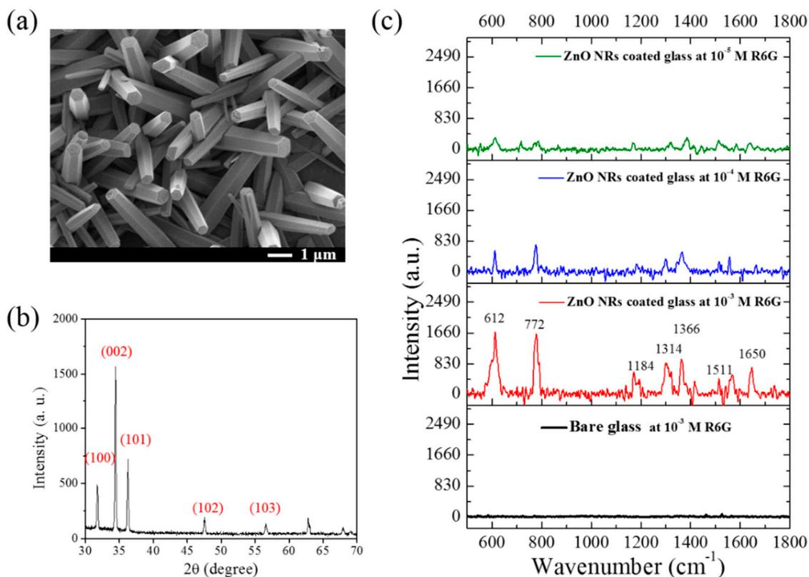
**Figure 2.** (a) SEM image of ZnO NRs fabricated using the sol–gel method on a glass substrate; (b) XRD patterns of ZnO NRs fabricated by the unannealed seed layer, indicating both vertical (002) and horizontal (100) and (101) growth direction; (c) Raman signal of rhodamine 6G (R6G) using bare glass and ZnO NR-coated glass as surface-enhanced Raman scattering (SERS) substrates.
