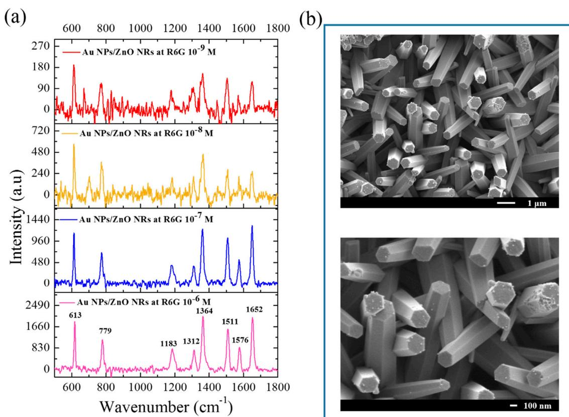
**Figure 6.** (a) Raman signal of R6G at different concentrations using Au-decorated ZnO NRs as the SERS substrate where the ZnO NRs was fabricated using the unannealed seed layer; (b) corresponding SEM images of Au-decorated ZnO NRs of different magnification.
