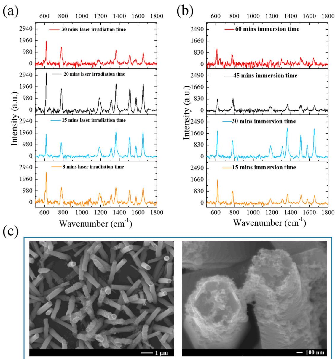
**Figure 7.** Raman signal of R6G ( $10^{-6}$  M) at various concentrations using Au-decorated ZnO NRs as the SERS substrate for AuNP fabrication for (a) different laser irradiation times at a fixed immersion time of 15 min and (b) different immersion time at a fixed laser irradiation time of 8 min during PLIP; (c) corresponding SEM images of Au-decorated ZnO NRs fabricated using an immersion time of 60 min.
