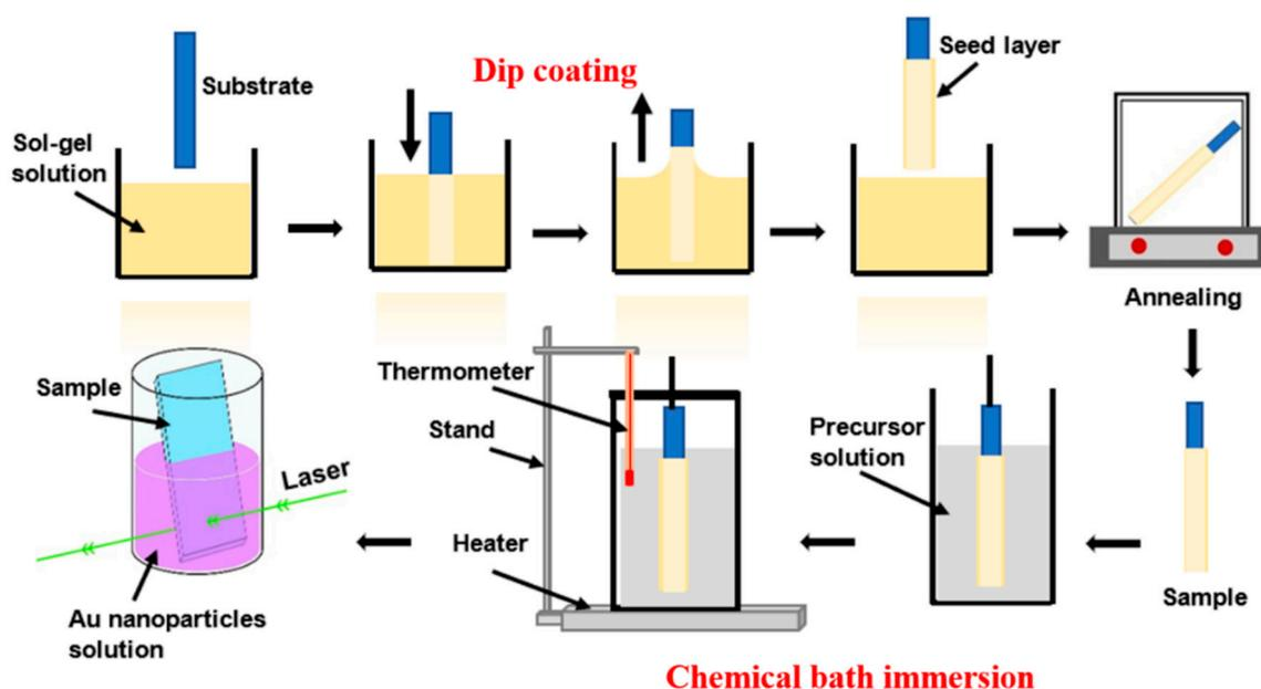
**Figure 1.** Schematic of fabricating surface-enhanced Raman scattering (SERS) substrate using zinc oxide (ZnO) nanorods (NRs) decorated with Au nanoparticles (AuNPs) synthesized through pulsed-laser-induced photolysis (PLIP).
