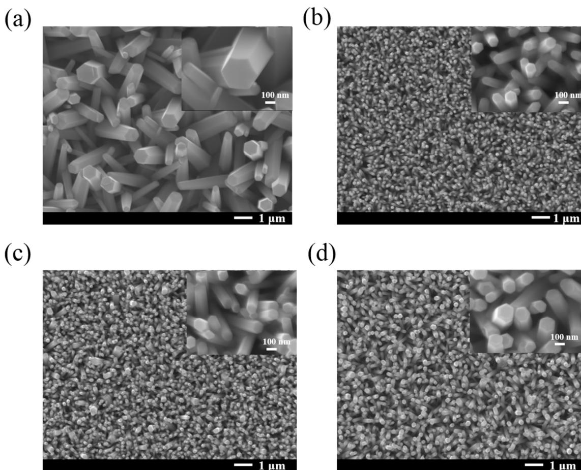
**Figure 4.** SEM images of ZnO NRs fabricated using seed layers annealed at (a) 100 °C, (b) 150 °C, (c) 200 °C and (d) 250 °C.
