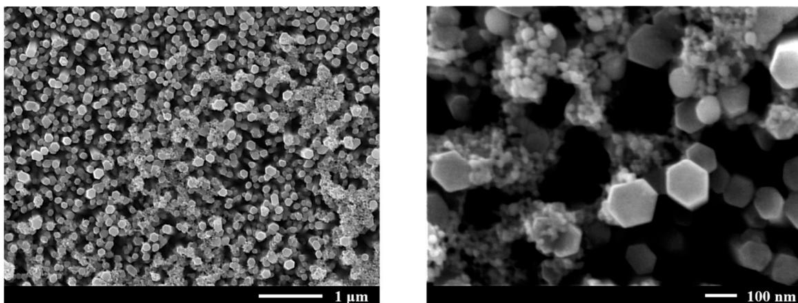
**Figure 5.** SEM images of Au-decorated ZnO NRs of different magnification.
