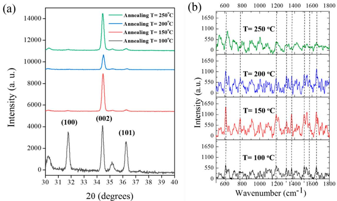
**Figure 3.** (a) XRD patterns of annealed ZnO NRs indicating the disappearance of horizontal (100) and (101) growth direction with the increase in the annealing temperature applied on the growth of seed layers; (b) Raman signal of R6G ( $10^{-3}$  M) using ZnO NR-coated glass as the SERS substrate, in which ZnO NRs were fabricated using seed layers annealed at different temperatures.
