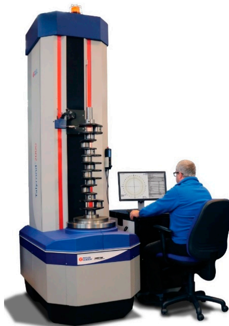
Figure 3. Talyrond 2000, an instrument with a rotary table for performing non-reference measurements of crankshaft geometry (courtesy of Taylor Hobson).
