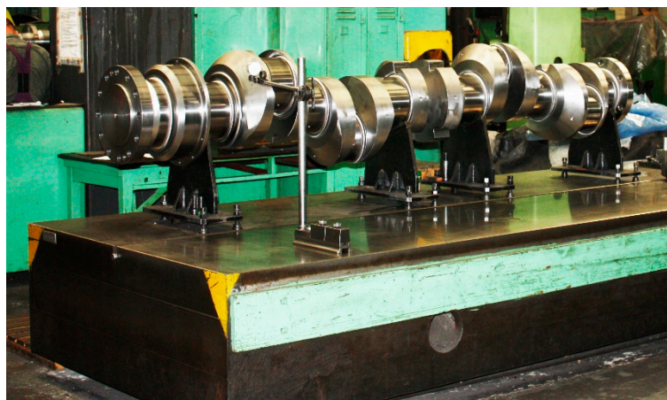
Figure 5. Measuring station for crankshafts for medium-speed engines.
