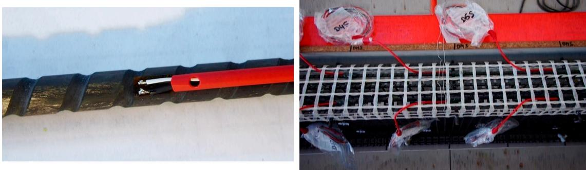
**Figure 4.** Left: Detail of internal strain gauge for carbon bar; right: position of strain gauges for FT01 in tension chord.
