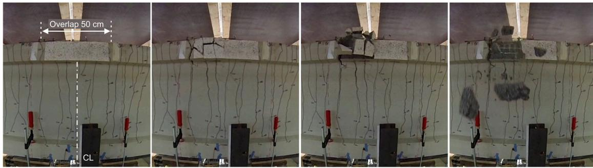
**Figure 10.** Failure sequence of FT03 in the overlap section in mid-span ( $\Delta t = 0.32$  s).
