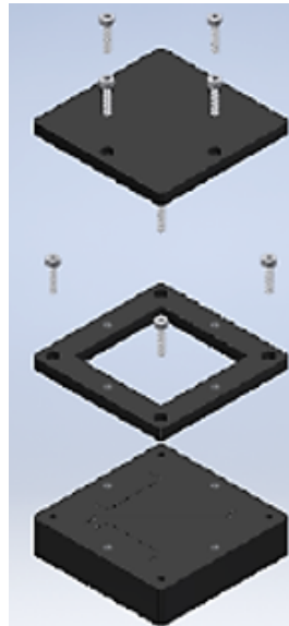
Figure 2. Computer-aided-design (CAD) magnetorheological-elastomer (MRE) mold with 3 layers: floor, middle, and top.
