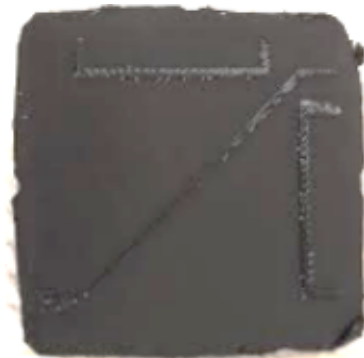
Figure 5. Manufactured 2-layer MR elastomer with nanoparticles.
