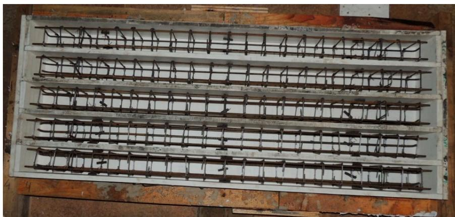
**Figure 1.** Beams before casting.
