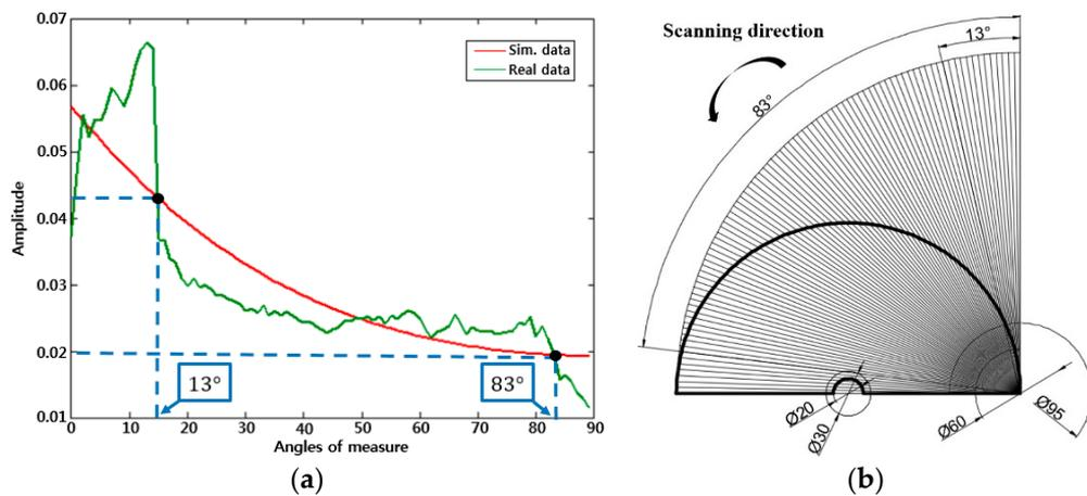
**Figure 22.** The attenuation curve of Lamb wave obtained from the experiment: (a) Attenuation curve; (b) Schematic of scanning direction.
