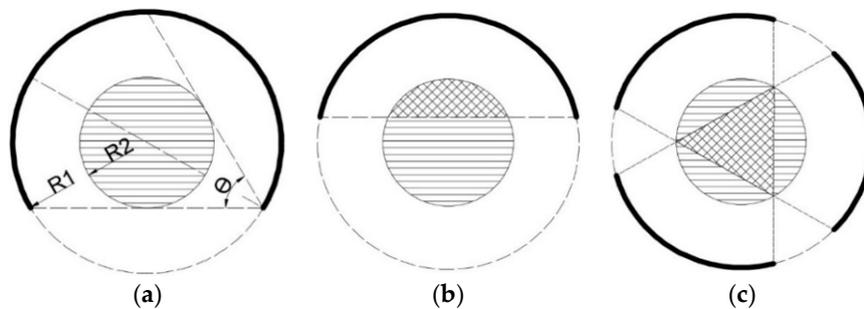
Figure 7. Schematic of the short-scan problem: (a) A conventional short-scan of  $\pi + \theta$  allows reconstruction of the whole object; (b) A continuous scan of less than  $\pi + \theta$  allows reconstruction of all object points inside the convex hull of the scan; (c) A scan of three equally spaced segments of  $80^\circ$  each allows reconstruction of a triangular ROI in the center of the object.
