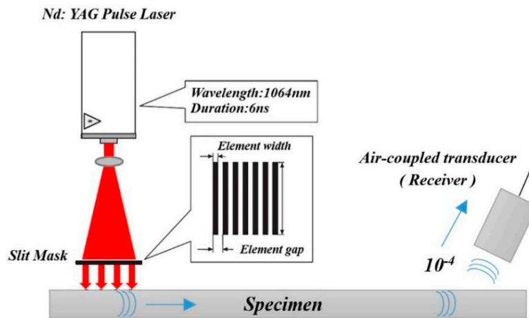
**Figure 9.** Improved transmission using a laser source. Values shown are approximate fractions of the original energy.
