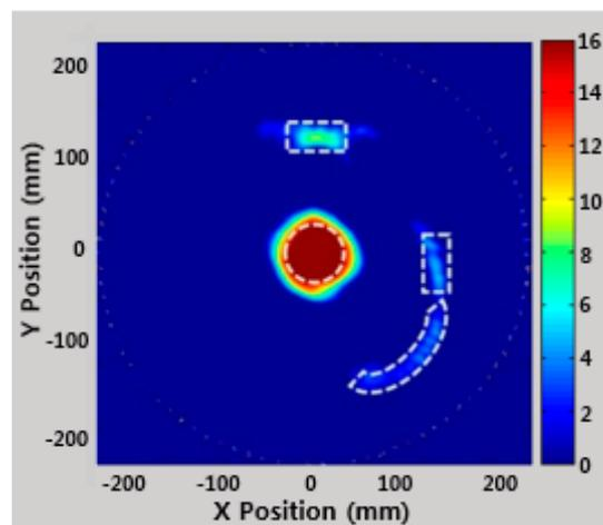
**Figure 26.** Multidefect imaging using the DHB algorithm.
