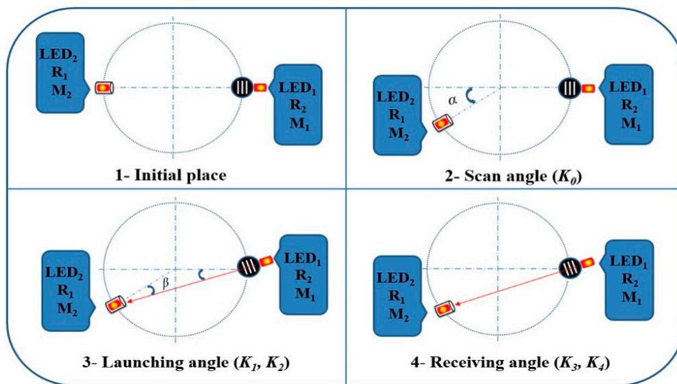
Figure 14. Schematic of the automatic scanning robot arm.
