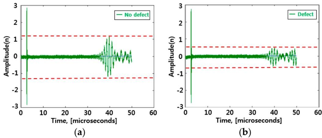
Figure 3. Guided wave signal: (a) No defect signal; (b) Defect signal.
