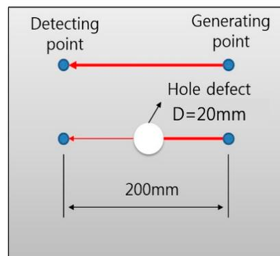
Figure 20. The schematic of the defect-detecting experiment.
