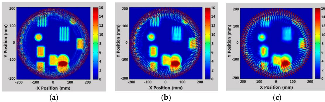
Figure 4. Simulated results from the filtered back projection (FBP) algorithm: (a) 180 Points; (b) 120 Points; (c) 90 Points.
