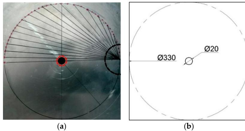
**Figure 23.** Circular defect specimen #1: (a) Circular defect specimen; (b) Circular defect specimen drawing (Unit: mm).
