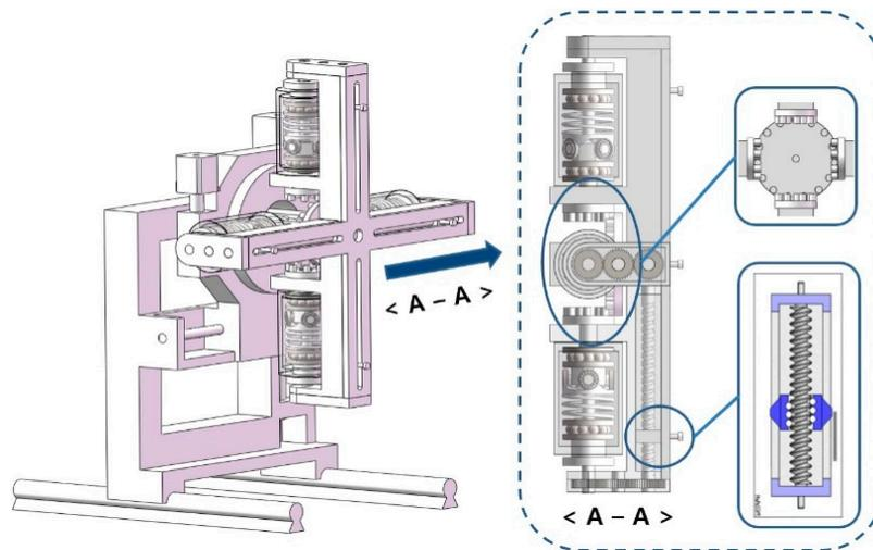
**Figure 17.** The 3-D model of the automatic clamping robot arms.
