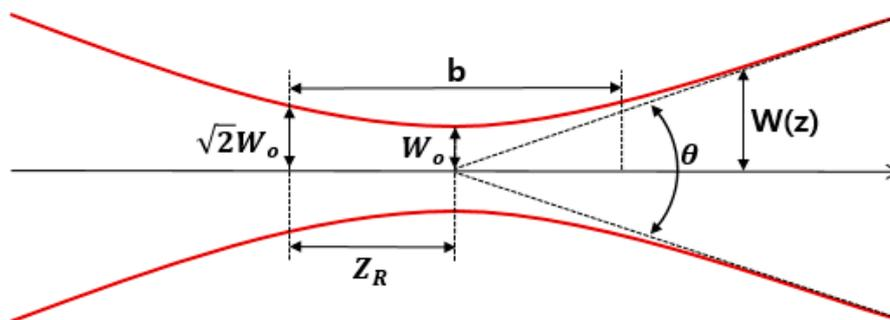
Figure 13. Gaussian beam propagation factor.
