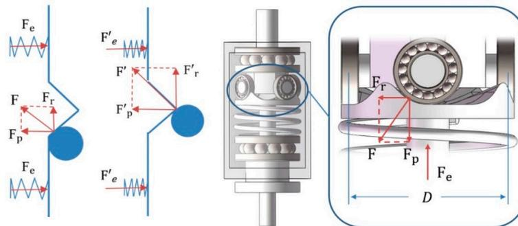
**Figure 18.** The force analysis of the automatic clutch.
