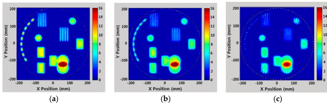
Figure 6. Simulated result from the Difference Hilbert Back Projection (DHB) algorithm: (a) 180 Point; (b) 120 Point; (c) 90 Point.
