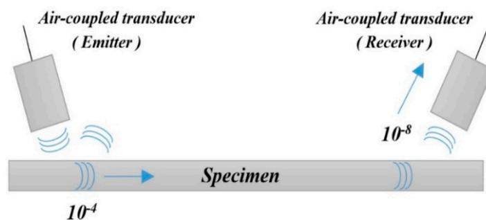
**Figure 8.** Transmission in air using two air-coupled transducers. Values shown are approximate fractions of the original energy.
