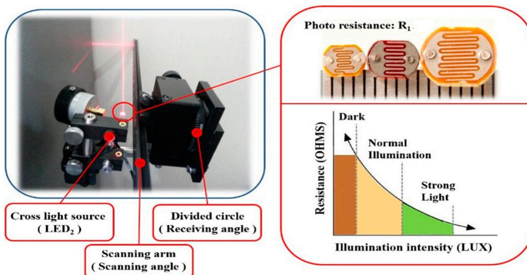
Figure 16. The actual settings of the automatic scanning robot arm.
