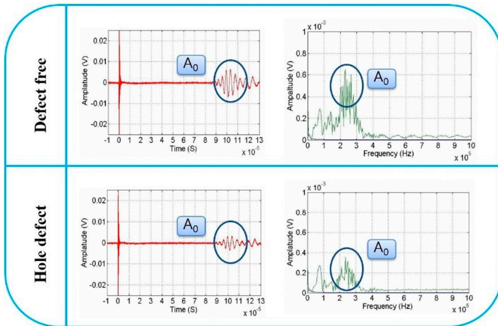
**Figure 21.** The signals of the defect detecting experiment.
