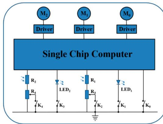
Figure 15. The working principle of the automatic scanning robot arm.
