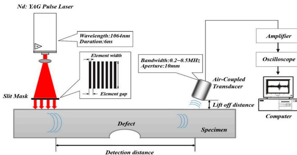
**Figure 12.** Schematic diagram of the experimental setup.
