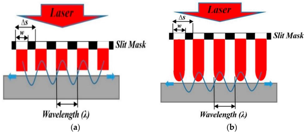
**Figure 10.** Schematic of the line laser sources of 1-D and Gaussian model: (a) One-dimensional theory; (b) Gaussian model.
