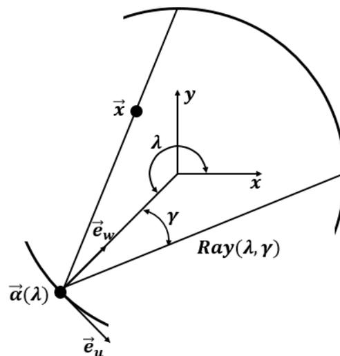
Figure 5. Fan-beam geometry based on the equiangular rays.
