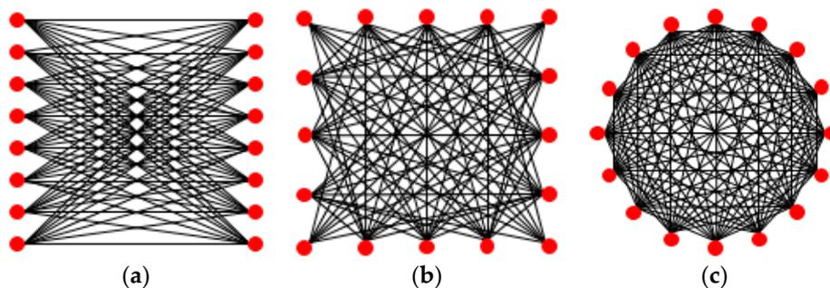
Figure 2. Three common iterative reconstruction methods: (a) Crosshole; (b) Double-crosshole; (c) Fan-beam.
