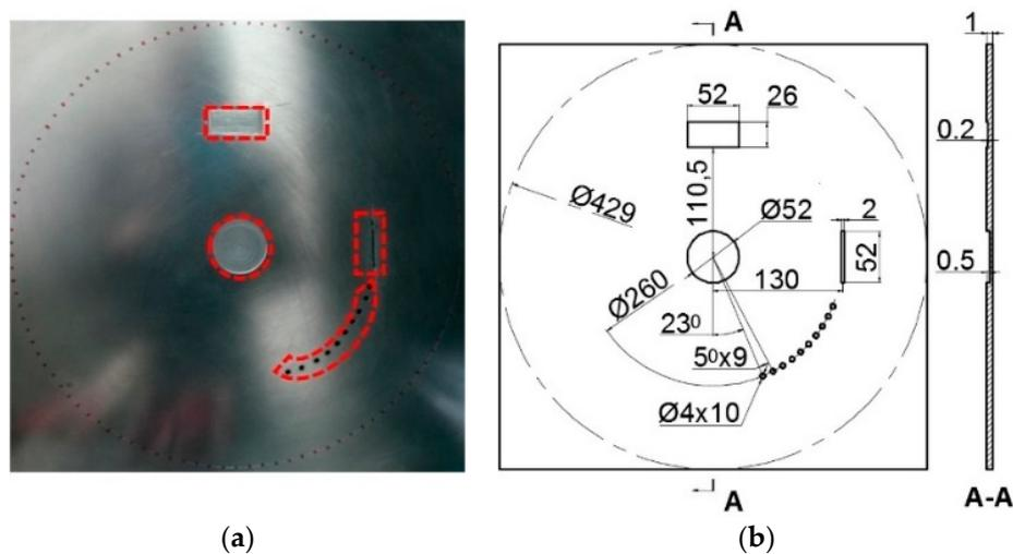
**Figure 25.** Image reconstruction of specimen #2: (a) Multidefect specimen; (b) Multidefect specimen drawing (Unit: mm).
