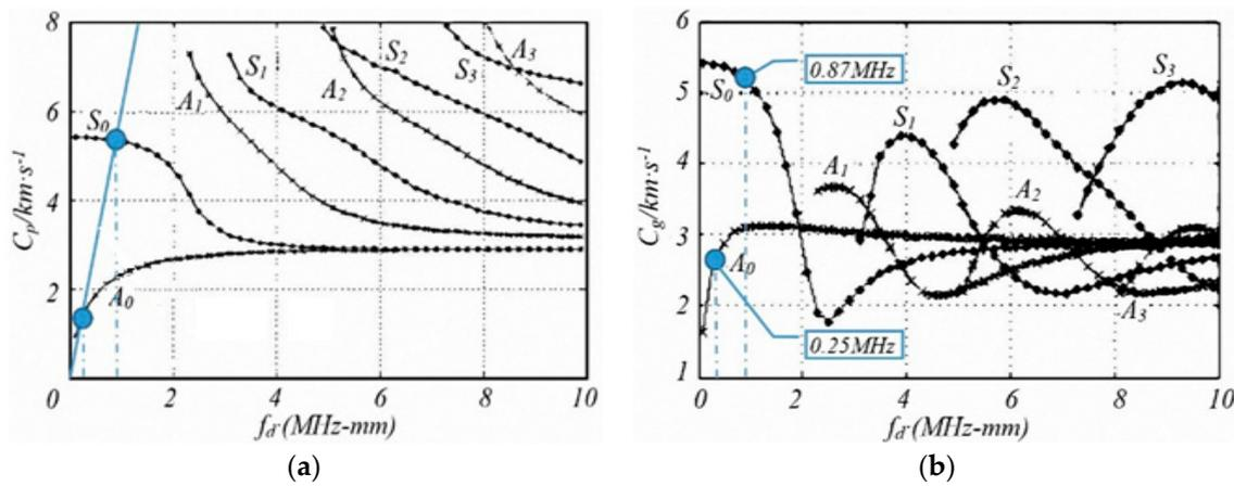
**Figure 11.** The frequency dispersion curve of a Lamb wave and the corresponding parameters: (a) Phased velocity; (b) Group velocity.
