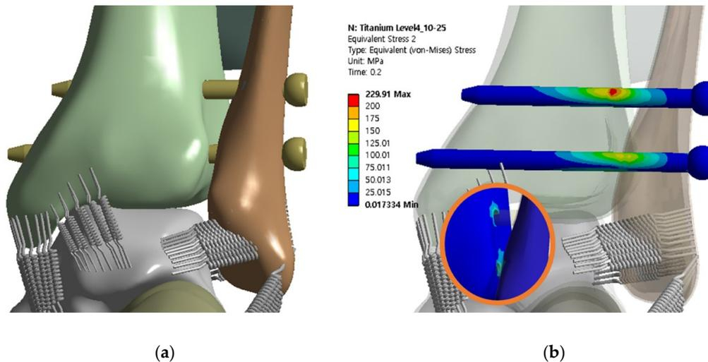
**Figure 15.** Finite element model and distribution of maximum equivalent stress with screws inserted at levels of 10 and 25 mm: (a) finite element model of syndesmotic fixation with double screws, and (b) maximum equivalent stresses of the screws and adjacent bone.
