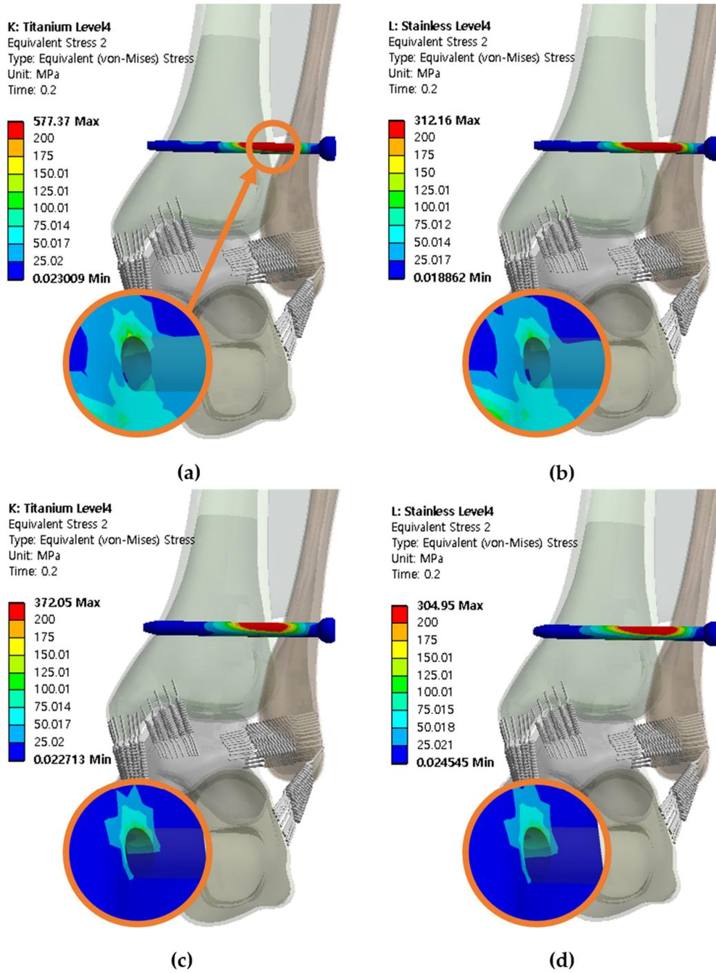
**Figure 5.** The von Mises stresses of the syndesmotomic screw and adjacent bone at screw level of 25 mm with four cortical bones purchased: (a) titanium screw with a diameter of 3.5 mm, (b) stainless steel with a diameter of 3.5 mm, (c) titanium screw with a diameter of 4.5 mm, and (d) stainless steel screw with a diameter of 4.5 mm.
