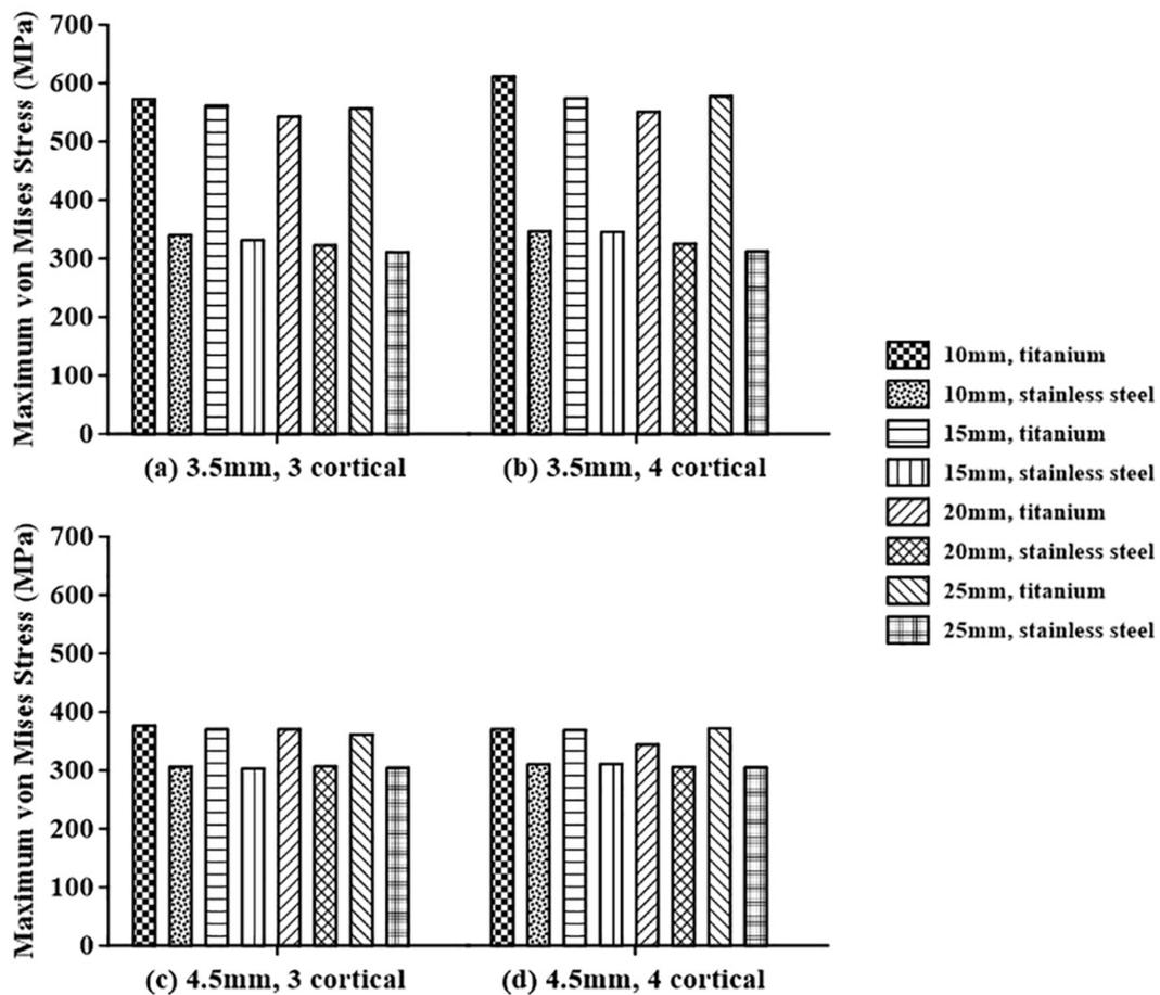
**Figure 6.** Analysis of the maximum von Mises stresses of the syndesmotic screw in terms of the syndesmotic screw material for screws with diameters of: (a) 3.5 mm penetrating three cortical bones, (b) 3.5 mm penetrating four cortical bones, (c) 4.5 mm penetrating three cortical bones, and (d) 4.5 mm penetrating four cortical bones.
