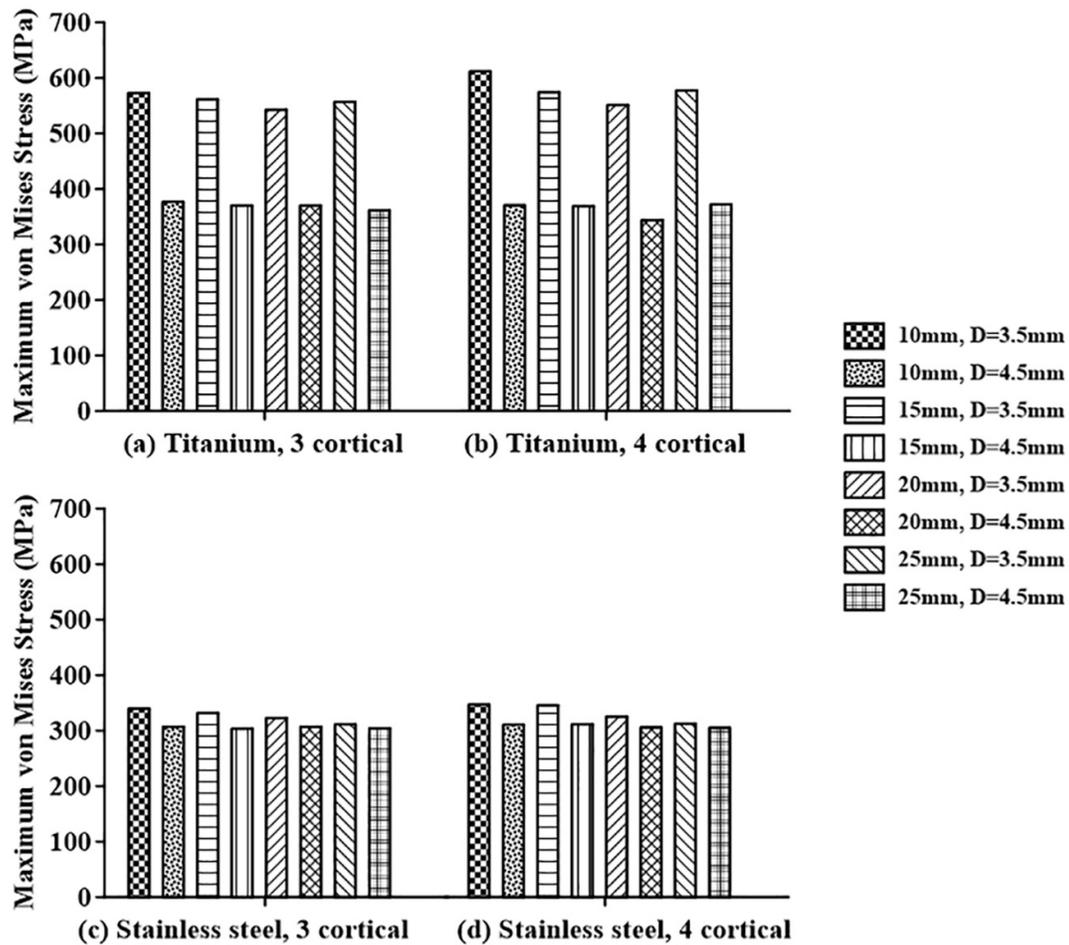
**Figure 7.** Analysis of the maximum von Mises stresses of the syndesmotic screw in terms of the diameter of the syndesmotic screw for: (a) titanium screw penetrating three cortical bones, (b) titanium screw penetrating four cortical bones, (c) stainless steel screw penetrating three cortical bones, and (d) stainless steel screw penetrating four cortical bones.
