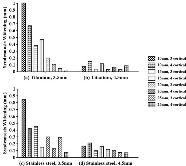
**Figure 14.** Analysis of the syndesmosis widening in terms of the number of penetrated cortical bones: (a) titanium screw with a diameter of 3.5 mm, (b) titanium screw with a diameter of 4.5 mm, (c) stainless steel screw with a diameter of 3.5 mm, and (d) stainless steel screw with a diameter of 4.5 mm.
