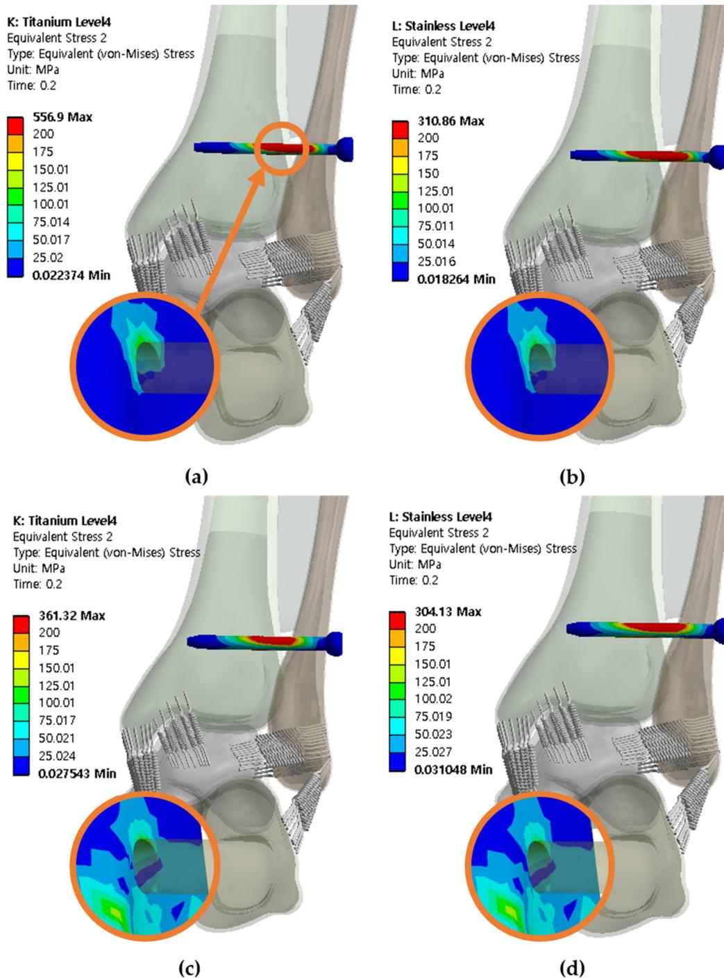
**Figure 4.** The von Mises stresses of the syndesmotic screw and adjacent bone at screw level of 25 mm with three cortical bones purchased: (a) titanium screw with a diameter of 3.5 mm, (b) stainless steel screw with a diameter of 3.5 mm, (c) titanium screw with a diameter of 4.5 mm, (d) stainless steel screw with a diameter of 4.5 mm.
