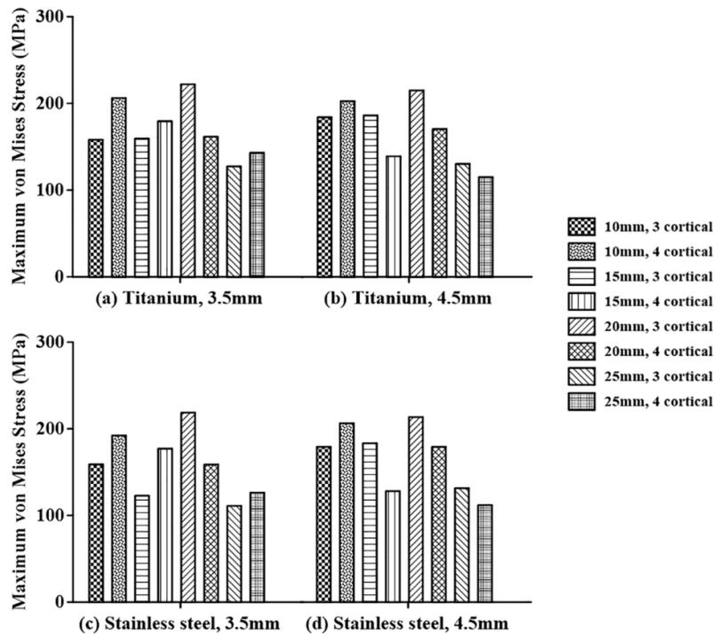
**Figure 11.** Analysis of the maximum von Mises stresses of the adjacent bone in terms of the number of penetrated cortical bones for: (a) titanium screw with a diameter of 3.5 mm, (b) titanium screw with a diameter of 4.5 mm, (c) stainless steel screw with a diameter of 3.5 mm, and (d) stainless steel screw with a diameter of 4.5 mm.
