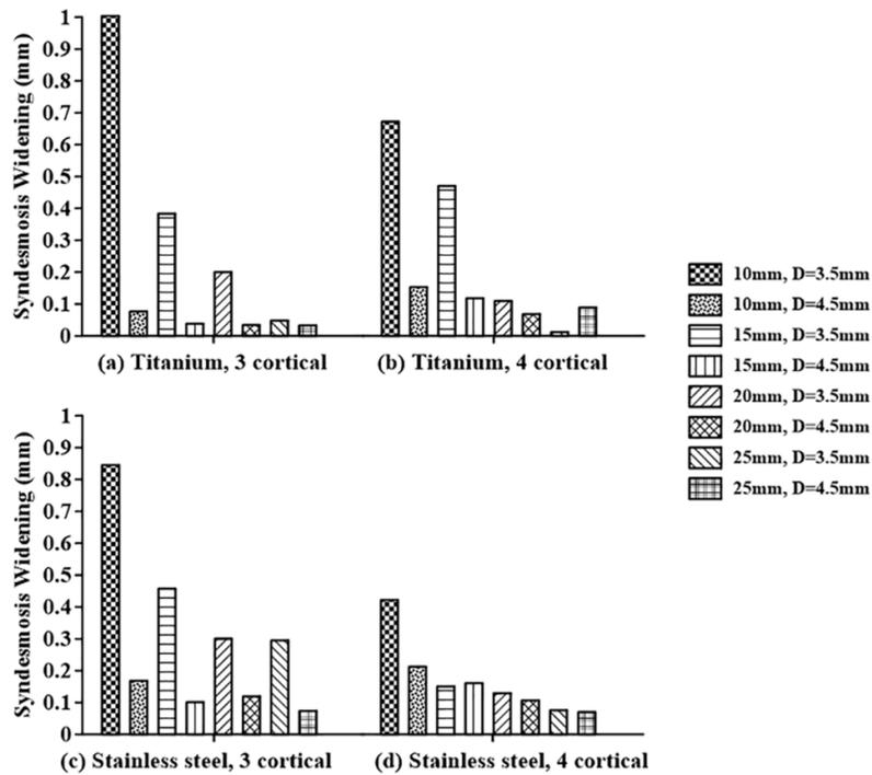
**Figure 13.** Analysis of the syndesmosis widening in terms of the screw diameter for: (a) titanium screw penetrating into three cortical bones, (b) titanium screw penetrating into four cortical bones, (c) stainless steel screw penetrating into three cortical bones, and (d) stainless steel screw penetrating into four cortical bones.
