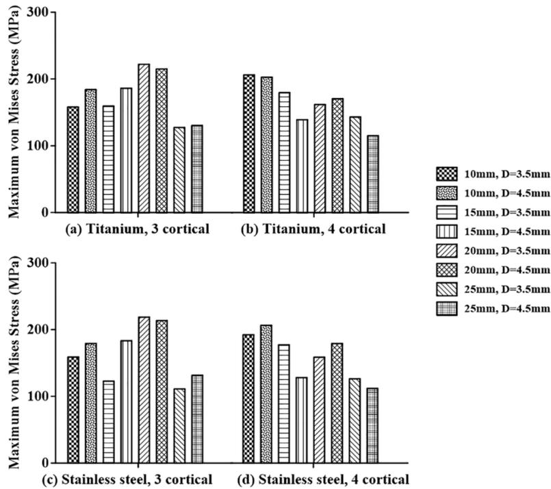
**Figure 10.** Analysis of the maximum von Mises stresses of the adjacent bone in terms of the diameter of the screw for: (a) titanium screw penetrating three cortical bones, (b) titanium screw penetrating four cortical bones, (c) stainless steel screw penetrating three cortical bones, and (d) stainless steel screw penetrating four cortical bones.
