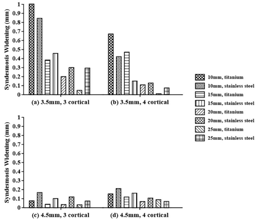
**Figure 12.** Analysis of the syndesmosis widening in terms of the screw material for screws with diameters of: (a) 3.5 mm penetrating into three cortical bones, (b) 3.5 mm penetrating into four cortical bones, (c) 4.5 mm penetrating into three cortical bones, and (d) 4.5 mm penetrating into four cortical bones.
