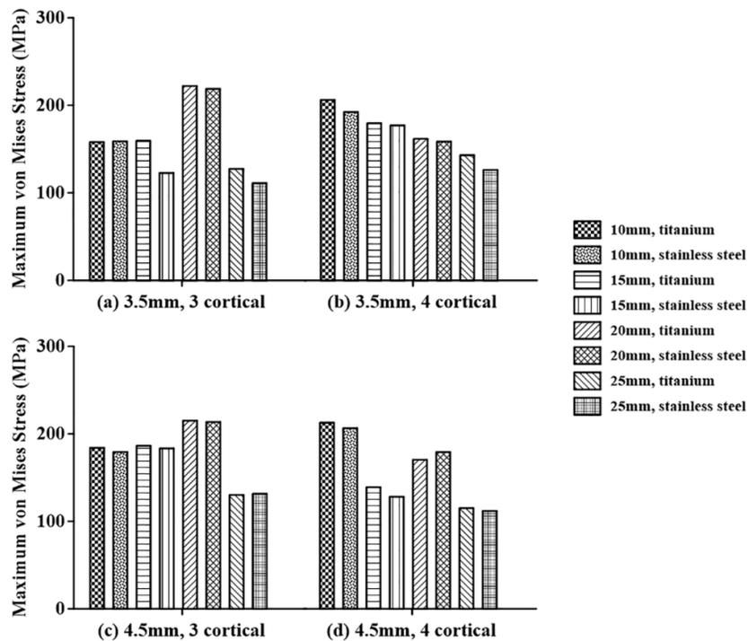
**Figure 9.** Analysis of the maximum von Mises stresses of the adjacent bone in terms of the screw material for screws with diameters of: (a) 3.5 mm penetrating three cortical bones, (b) 3.5 mm penetrating four cortical bones, (c) 4.5 mm penetrating three cortical bones, and (d) 4.5 mm penetrating four cortical bones.
