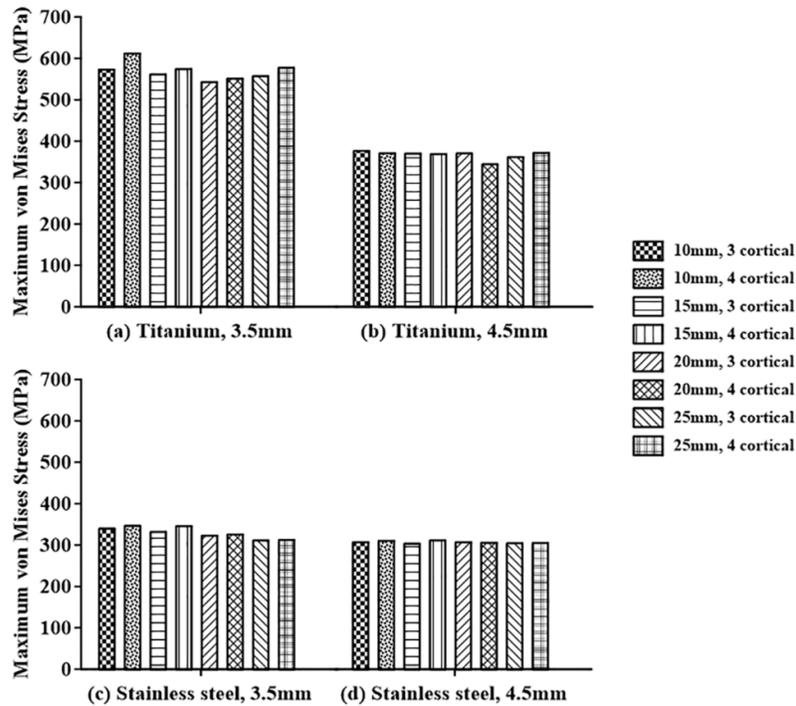
**Figure 8.** Analysis of the maximum von Mises stresses of the syndesmotic screw in terms of the number of penetrated cortical bones for: (a) titanium screw with a diameter of 3.5 mm, (b) titanium screw with a diameter of 4.5 mm, (c) stainless steel screw with a diameter of 3.5 mm, and (d) stainless steel screw with a diameter of 4.5 mm.
