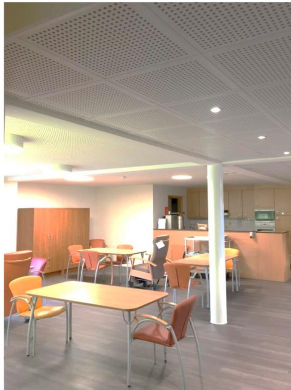
**Figure 5.** Picture of the nursing home (NH) living room after the installation of the acoustic floating floor and absorbing ceilings.
