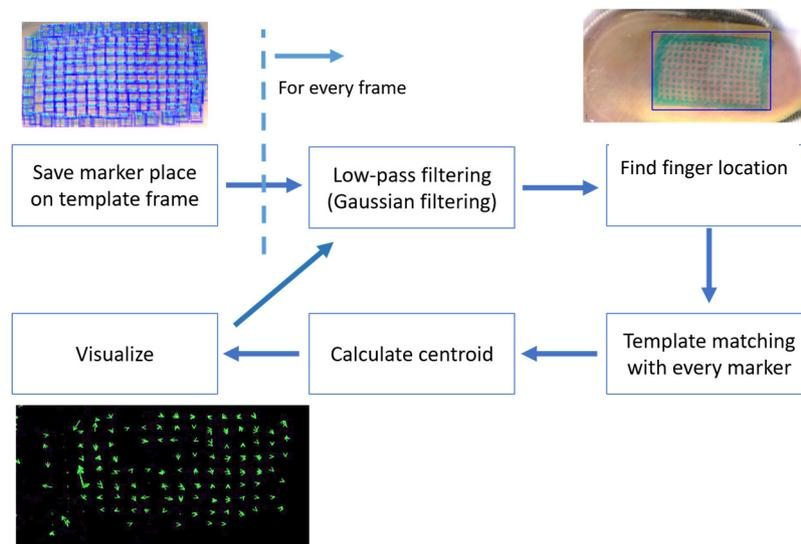
**Figure 7.** Flow of the image-processing algorithm.
