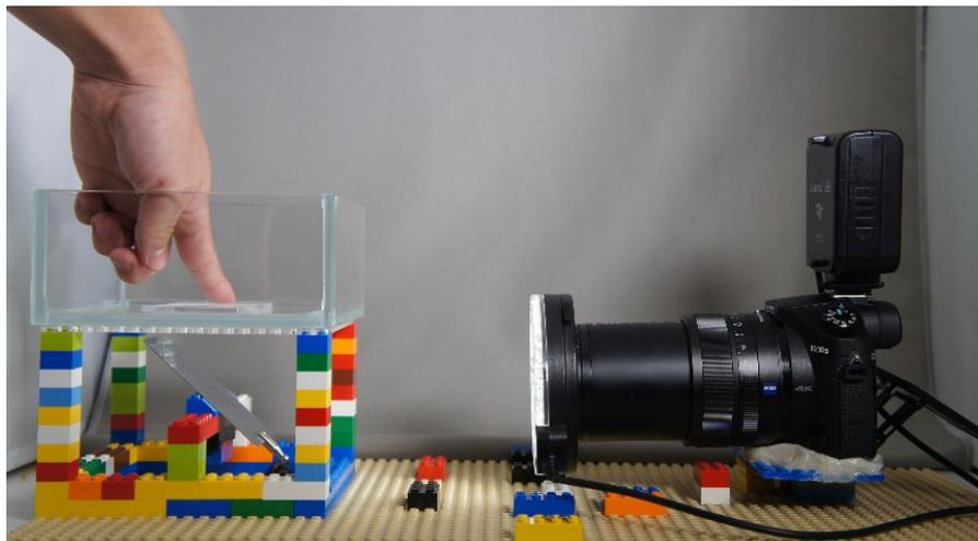
**Figure 4.** View of the measurement system taken from the side. To verify the principle of the system, we implemented a measurement system using Lego blocks. The texture is made optically transparent by filling an aquarium with a silicone oil having the same refractive index as the texture.
