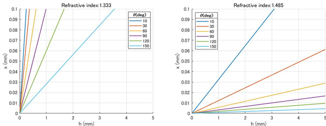
**Figure 3.** Relationship between distance from the refractive point to the skin ( $h$ ) and optical misalignment ( $x$ ) when using silicone oil (left) and water (right). Each line in the graph shows the relationship when the texture angle is changed.
