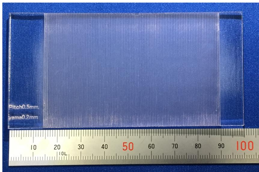
**Figure 9.** Textured surface used for the experiment. Pitch width: 0.6 mm.
