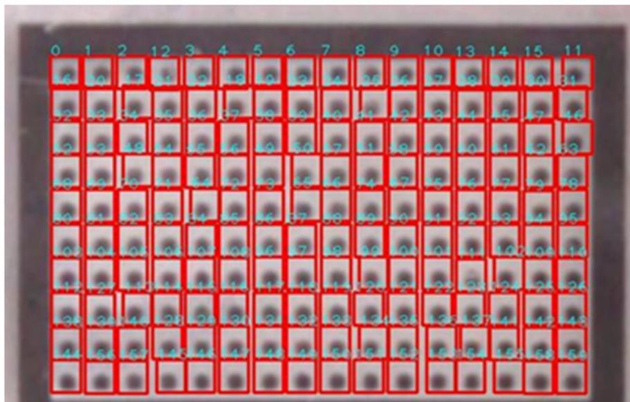
**Figure 10.** The result of marker recognition. The image is blurred because the Gaussian filter has been applied. A red square indicates that the program recognized that area as a marker. A video of the the measurement video (Video S1) is presented in Supplementary Materials.
