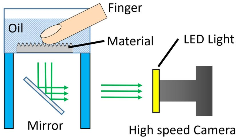
**Figure 5.** Overview of the experimental setup. By filling the water tank with oil, the texture is optically transmitted. The camera is placed in front of a mirror to observe fingertips through the textures, and the LED is attached to reduce the noise from the high-speed camera.
