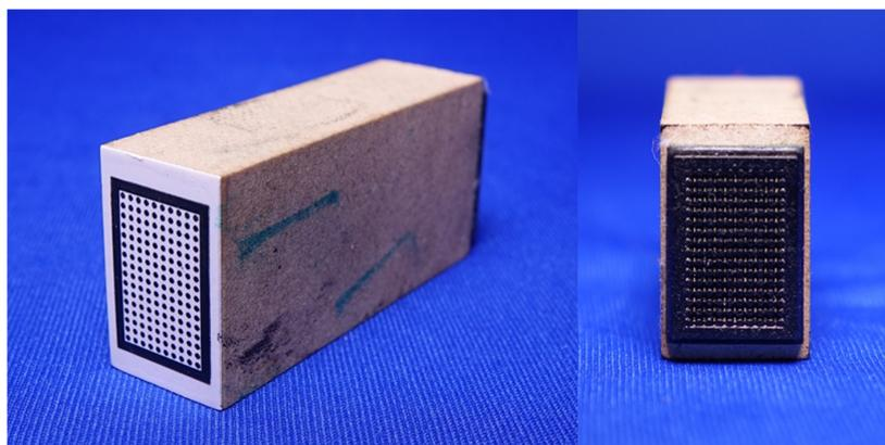
**Figure 6.** Stamp used to apply the markers to the finger. Points were placed in a  $10 \times 16$  array, each having a 0.5 mm diameter and 1.0 mm center-to-center intervals.
