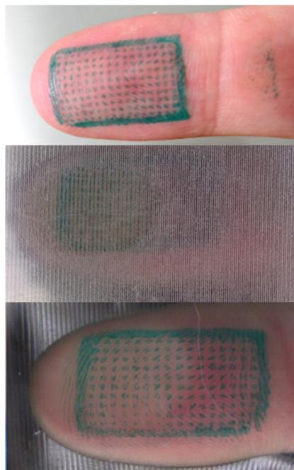
**Figure 1.** Top: fingertip with markers; middle: fingertip viewed through the textured surface without oil; bottom: fingertip viewed through the textured surface submerged in oil.
