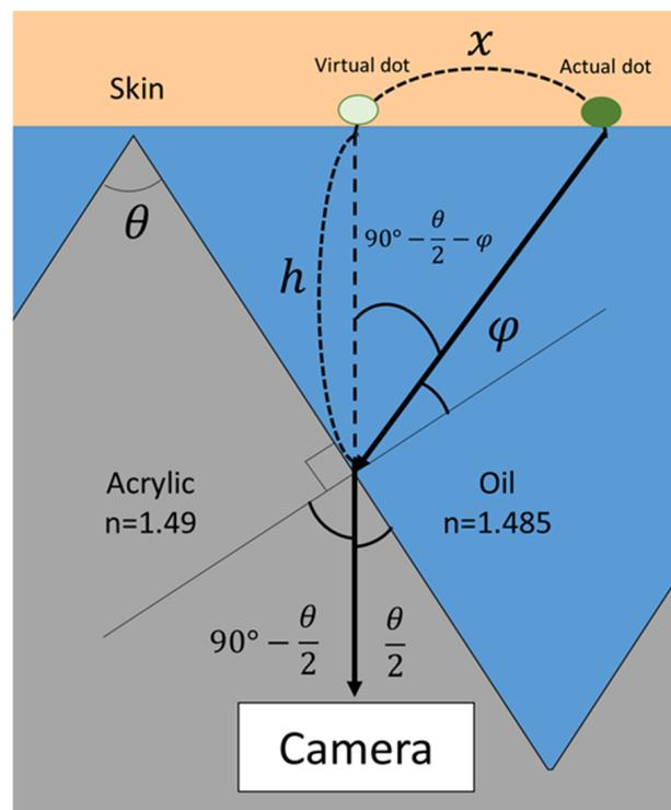
**Figure 2.** Overview of light refraction and the amount of optical misalignment caused by it. The refractive index of the medium, the angle of the texture, and the distance to the fingertip are defined as  $n$ ,  $\theta$ , and  $h$ , respectively. As temporary variables, the angle of incidence and the amount of optical deviation from the actual dot are set to  $\varphi$  and  $x$ , respectively.
