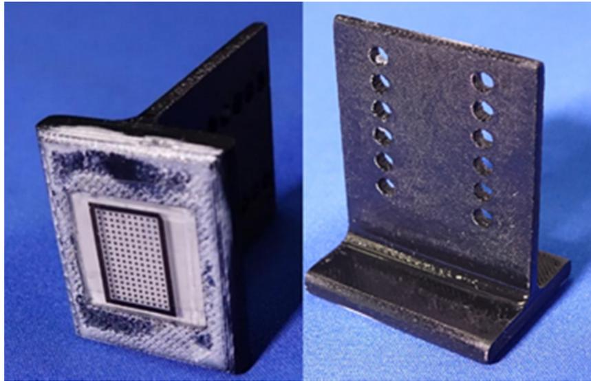
**Figure 8.** Artificial finger with markers printed on oil-proof paper.
