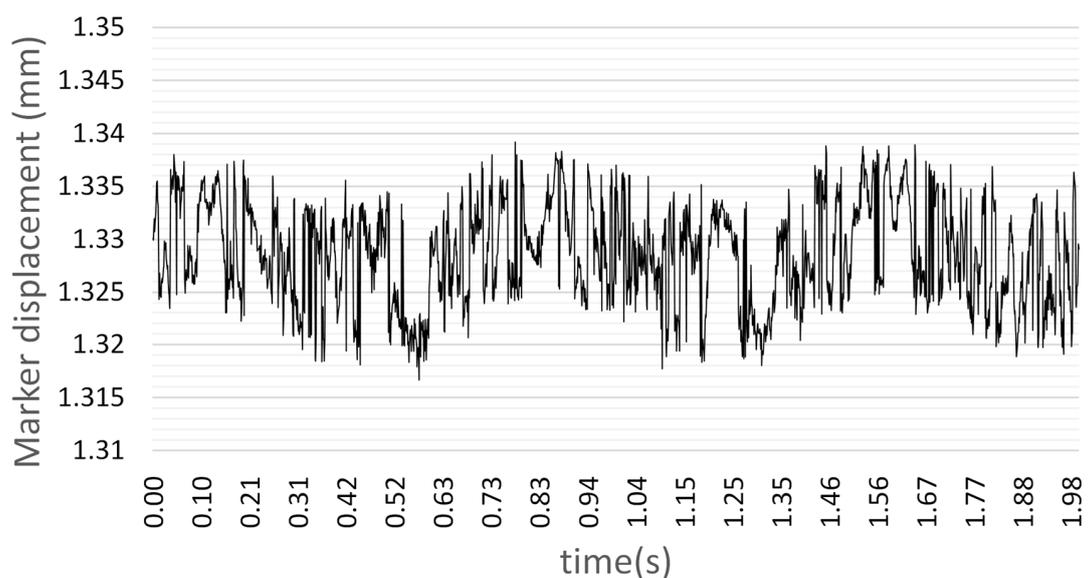
**Figure 11.** Displacement of the No. 0 marker in the slope direction from Figure 10. The variation generated by this measurement is noise. This is because there is no variation between the markers in this measurement. It can be seen that the average noise level in this marker is 20  $\mu\text{m}$ .
