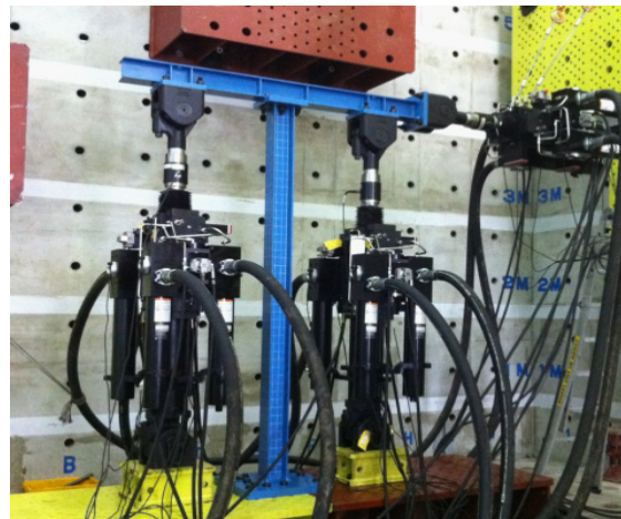
Figure 6. Test set-up for steel frame and actuators.
