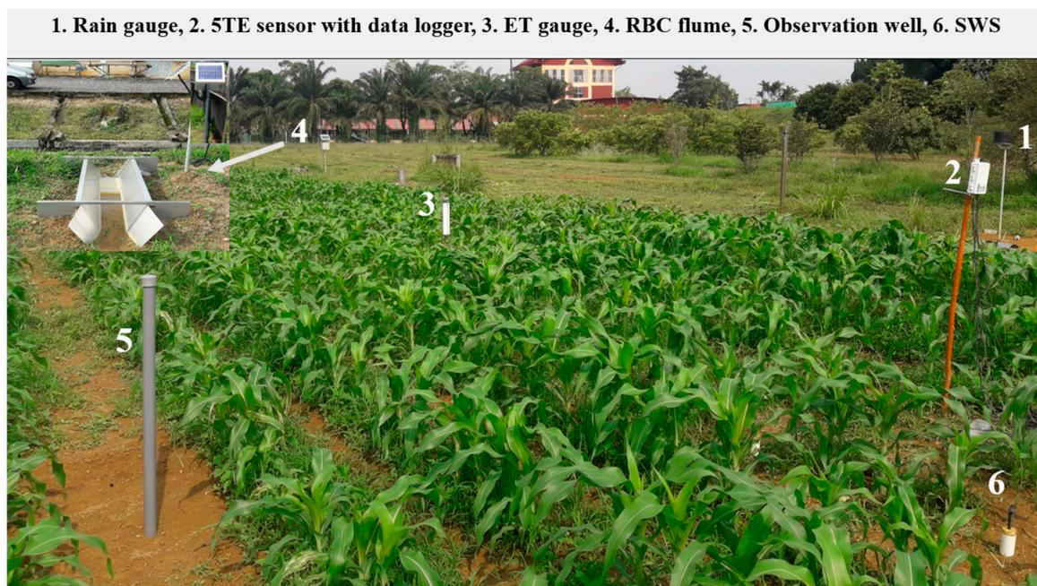
**Figure 2.** A view of the installation of different equipment in the field.
