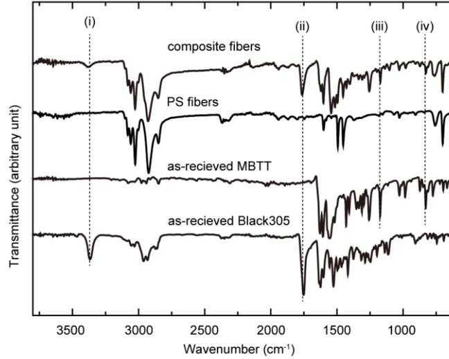
Figure S2: ATR-FTIR spectra of the composite fibers, MBTT (photoacid), leuco dye Black 305, and PS fibers.
