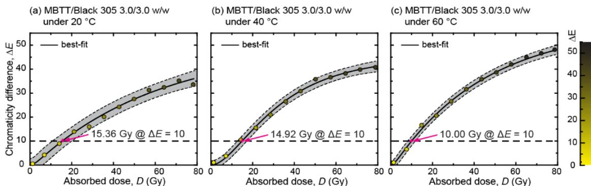
Figure S4. Dose-response curves of the fibrous color dosimeters made of the composite fibers consist of MBTT/Balck305 3.0/3.0 by weight at different temperatures (a) 20, (b) 40, (c) 60 °C. The color bar signifies the color tone corresponding to  $\Delta E$ . The black broken line indicates the point at which color change can be visually observed.
