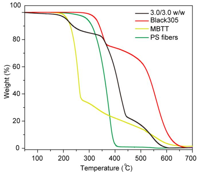
Figure S3: TGA thermograms of the fibrous color dosimeter with MBTT/Black305 ratio at 3.0/3.0 w/w, Black305, MBTT, and PS fibers in air.
