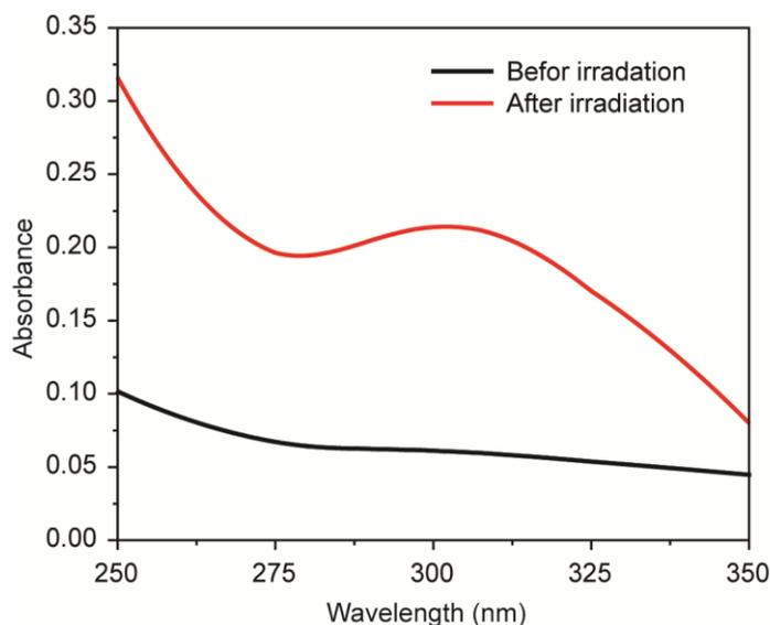
Figure S1: Absorbance spectra of the Fricke dosimeter before and after X-ray exposure.
